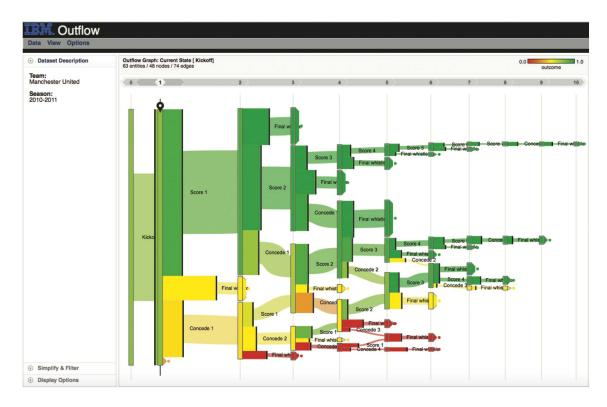
Figure 2.6: OutFlow [7] uses a network structure to aggregate similar event sequences into progression pathways and summarizes the pathways' possible outcomes.
