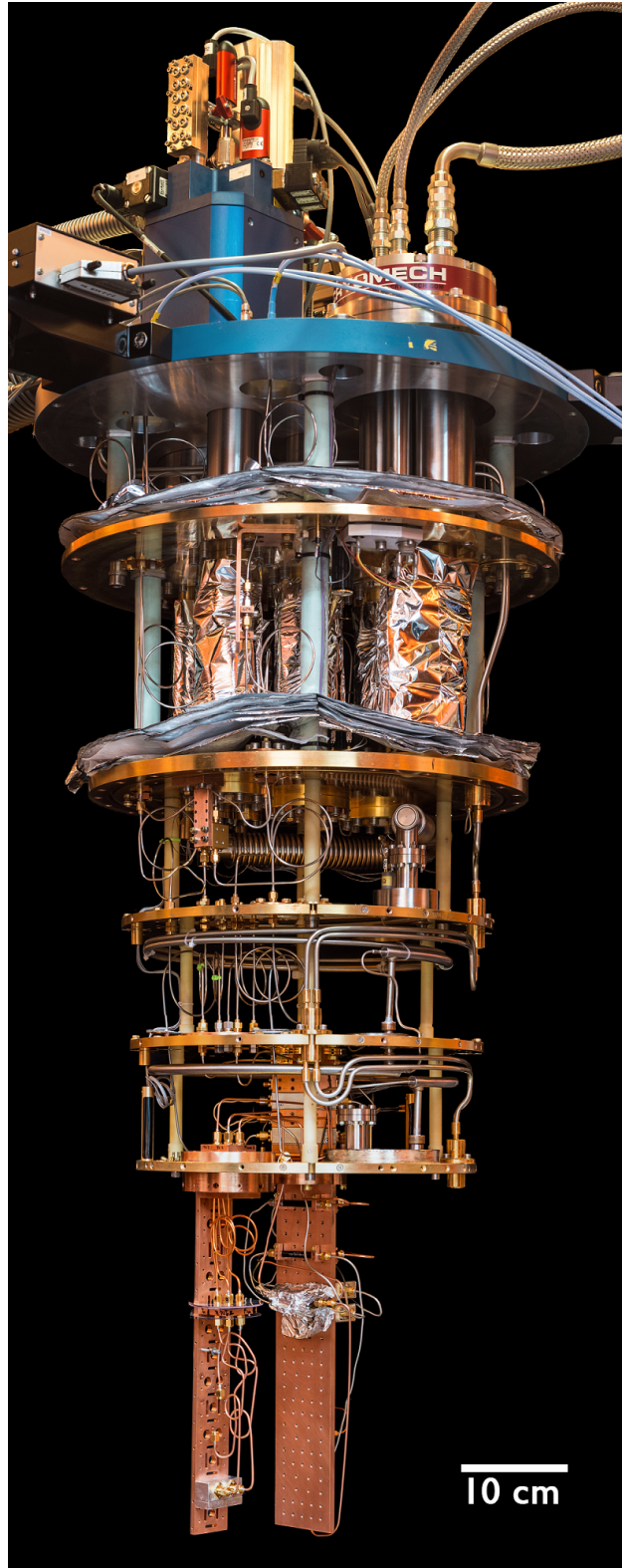
Fig. 4.1 Photograph of the CF-450 Dilution refrigerator with two Cu mounting posts. The thermal shields and cryoperm shields have been removed.
