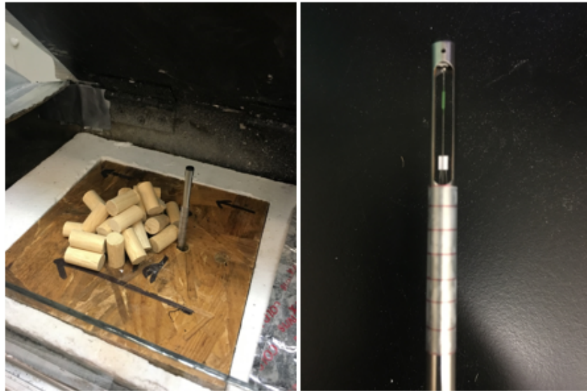
Figure 3.10: Photographs showing the methodology used to measure wind speeds including the tip of the hot-wire anemometer (right) and wind speed measurements being performed with a simulated presence of firebrands (left).
