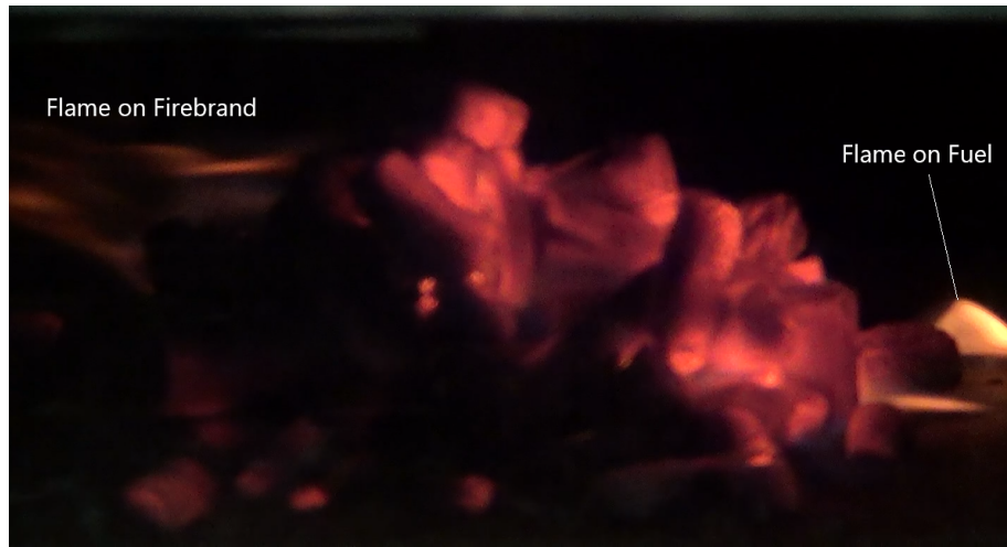
Figure 4.26: Photograph showing flames present both over the pile of firebrands and over the fuel surface.
