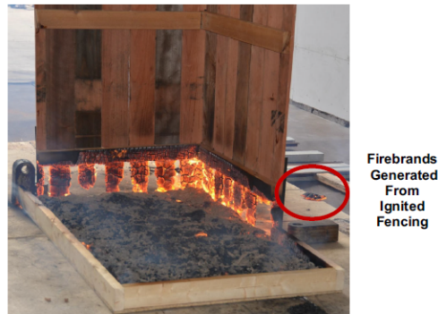
Figure 2.3: Flaming in the corner assemblies were additional fuel was presented. Also firebrand generated from fences can be seen. (From [2])
