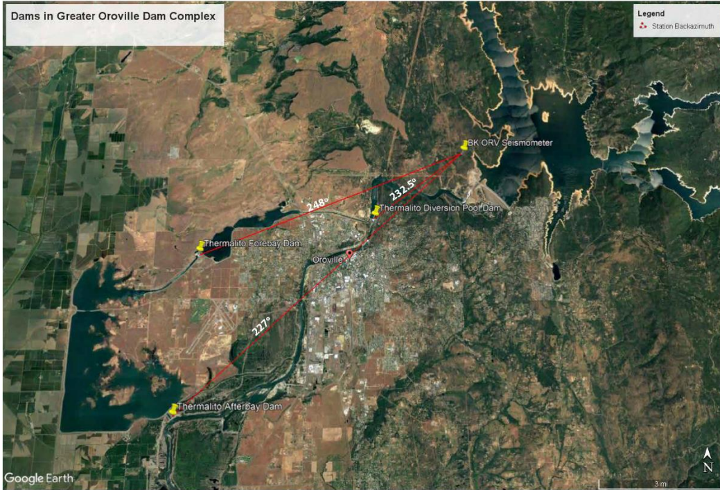
Figure S6- Three other dams- Thermalito Forebay Dam, Thermalito Diversion Pool Dam, and Thermalito Afterbay Dam- are a part of the Oroville Dam Complex and are at backazimuths of 248°, 232.5°, and 227°, respectively. The town of Oroville, California is located between station backazimuths of approximately 248° and 217°.
