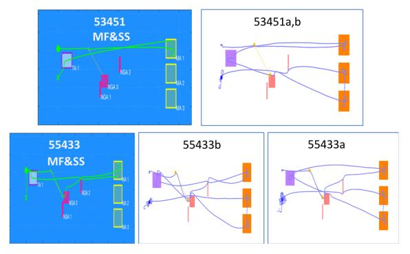
Figure 4.31: Boundary Pair 2 plots comparing the simulated result (left) to trajectory executed during in-water tests (right). Multiple blue lines are due to overlaying the results of all field tests on top of one another.
