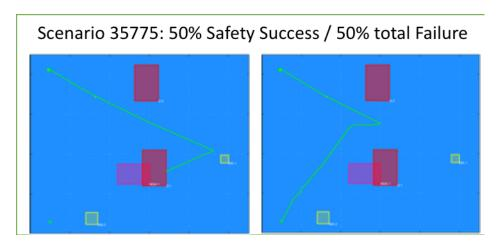
Figure 4.9: Example of multiple runs for a probabilistic scenario. Small inaccuracies in the position estimate can cause large changes in when it decides to return home.
