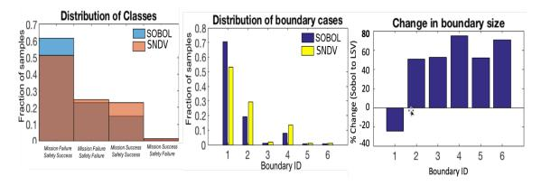
Figure 3.12: Results of the performance mode and boundary distributions for the Sobol and S-NDV search approaches executed on the UUV mission.
