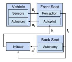
Figure 6.3: Flowchart outlining the autonomous vehicle testbed used for imitation learning.
