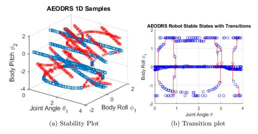
Figure 5.7: Scatter plots for the 1DOF AEODRS robot with only the shoulder joint actuated. (left) An isometric view showing how stable states in blue and unstable states in red. (right) A top down view with red arrows showing transitions between nodes.
