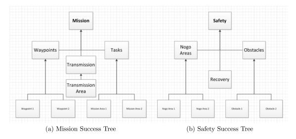
Figure 4.11: Diagram of the hierarchical score trees for our UUV simulation illustrating the first 3 levels of the score tree for both mission success and safety success.
