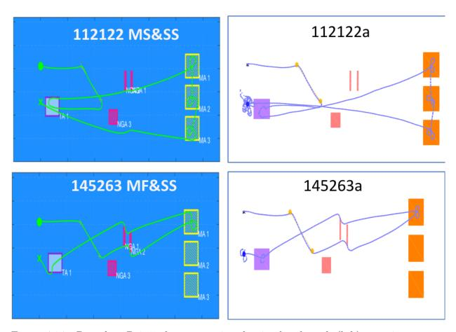
Figure 4.34: Boundary Pair 5 plots comparing the simulated result (left) to trajectory executed during in-water tests (right). Multiple blue lines are due to overlaying the results of all field tests on top of one another.
