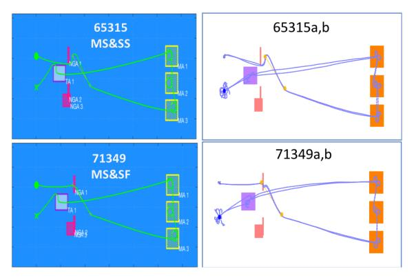
Figure 4.32: Boundary Pair 3 plots comparing the simulated result (left) to trajectory executed during in-water tests (right). Multiple blue lines are due to overlaying the results of all field tests on top of one another.
