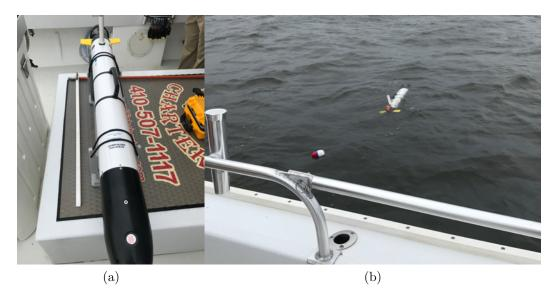
Figure 4.1: IVER UUV used for the on-water tests of the autonomous vehicle software. These photographs were taken during the hydrodynamic tests conducted in the Chesapeake Bay.
