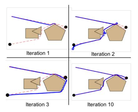
Figure 6.1: In this example scenario the imitator (blue line) rapidly converges to the expert agent's path (red line) despite never experiencing this scenario during training.
