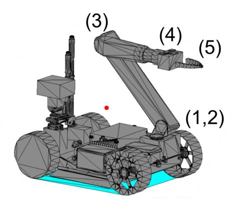
Figure 5.5: Illustration of the 5 DOF robot model. Its degrees of freedom are (1) Shoulder Yaw, (2) Shoulder Pitch, (3) Elbow angle, (4) Wrist rotation, (5) Jaw Angle
