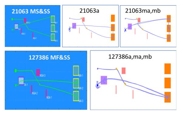
Figure 4.33: Boundary Pair 4 plots comparing the simulated result (left) to trajectory executed during in-water tests (right). Multiple blue lines are due to overlaying the results of all field tests on top of one another.
