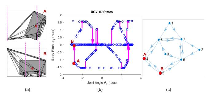
Figure 5.1: Overview of the stability framework. (a) Illustration of a robot with a single arm and 1 DOF tipping over (b) A state plot of the robot where blue markers represent states in C-space and magenta arrows showing where transitions occur. (c) A Node plot is created by compressing the stable regions of the state space into nodes and their transitions into edges.
