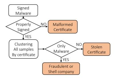
Figure 3.2: Flowchart of the abuse detection algorithm.
