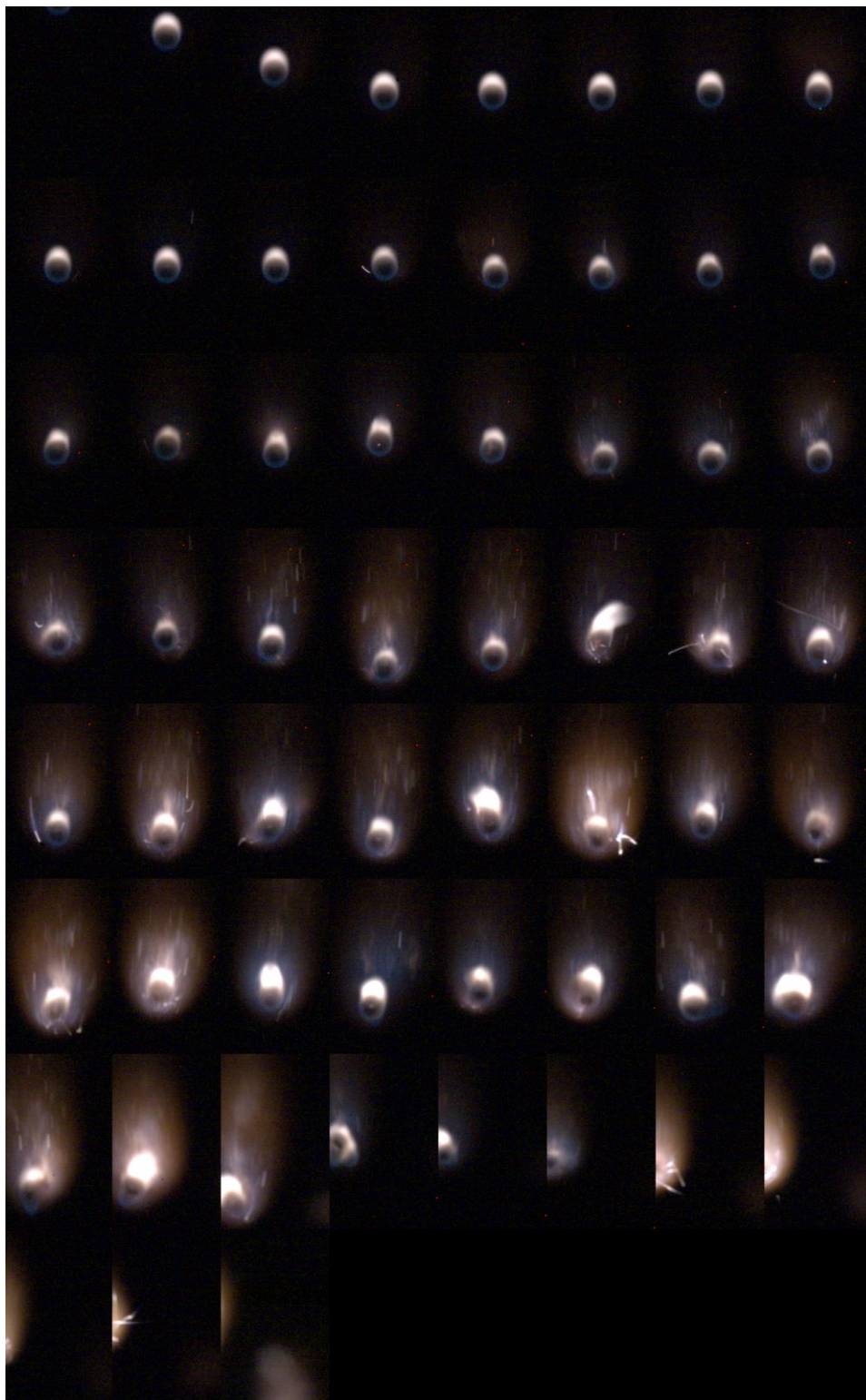
Figure C.18: nAl/AP/5%NC MPs in kerosene/TOPO. 141.5 ms of burning time is shown with 2.424 ms period. 3X brightness shown.
