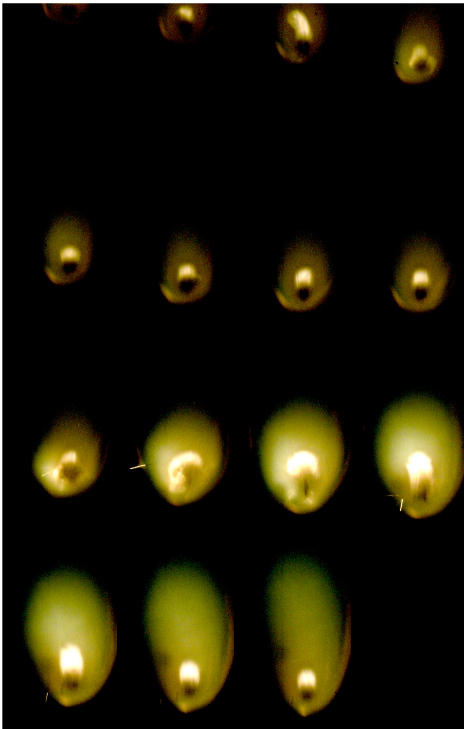
Figure C.4: nAl/CuO/5%NC MPs in kerosene/TOPO (Droplet C). 61.1 to 69.9 ms burning time shown with 0.303 ms period. 3X brightness shown.
