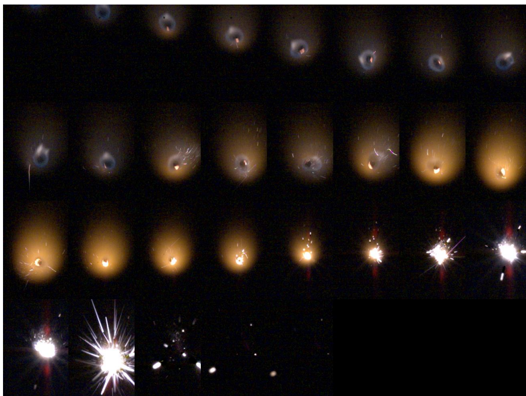
Figure C.21: n\text{Al}/\text{Al}_2\text{O}_3/5\%\text{NC} MPs in kerosene/TOPO. 30.6 ms of burning time is shown with 0.909 ms period. 3X brightness shown.
