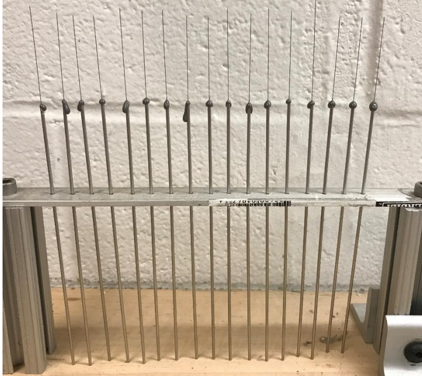
Figure D.19: Assembled needles in the drying rack
