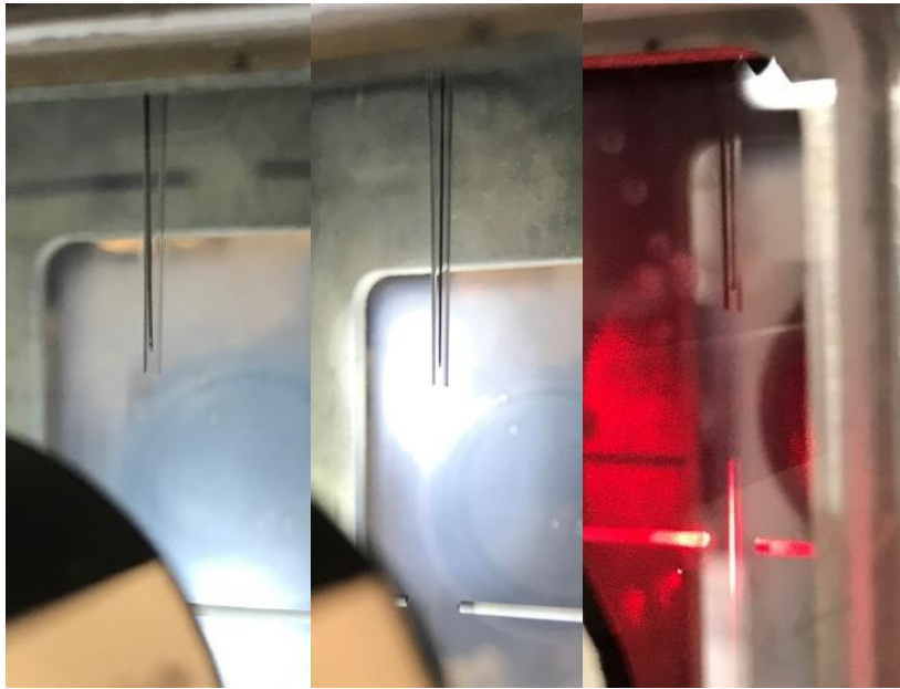
Figure D.7: Needle nested in the nozzle showing misalignment, alignment, and successful droplet generation
