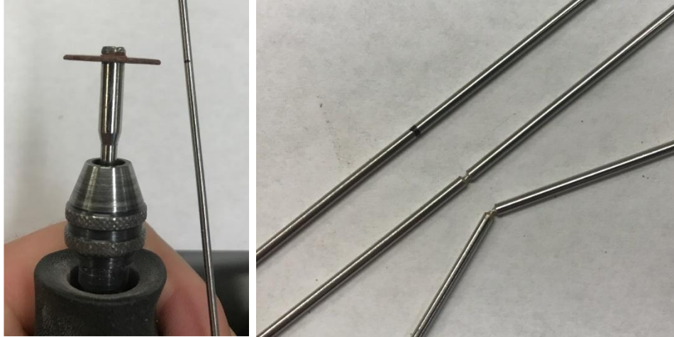
Figure D.14: Cutting of IDEX tubing in half by scoring and breaking.
