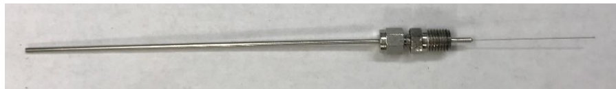
Figure D.6: Replacement needle in its mounting adapter with NPT end to the right
