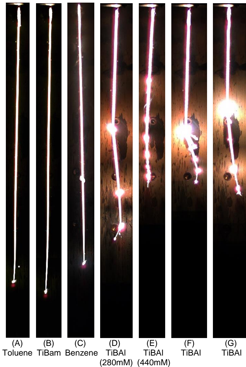
Figure 65: Representative time-lapse images of free-falling droplets combusting with and without 810 mM TiBAI additive or TiBam/Benzene control additives. (A) Pure Toluene, (B) 810 mM Triisobutylamine in Toluene, (C) 810 mM Benzene in Toluene, (D-E) Two types of disruptions from 810 Triisobutylaluminum in Toluene. The mid-height emission expansion in (C) is an artifact caused by reflection off a spot of residue on the experiment cover glass and is not a disruption.
