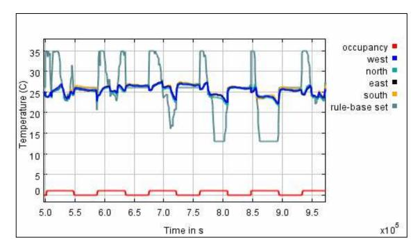
Figure 5.9: Profiles of room occupancy, rule-based setpoint, and temperature versus time (sec) for Control Case 1.
