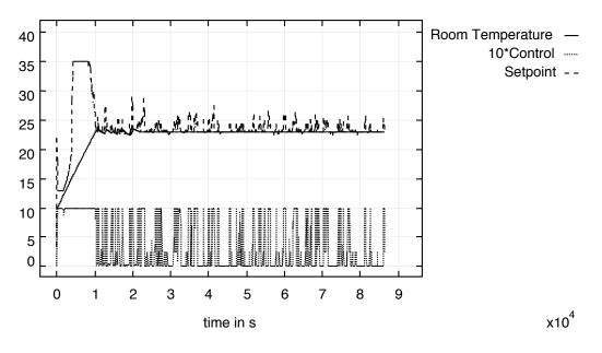
Figure 5.5: Setpoint, room temperature, and control signal.
