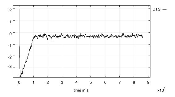
Figure 5.6: Dynamic thermal sensation model – Acceptable range is -0.5 <  $\rm DTS < 0.5$
