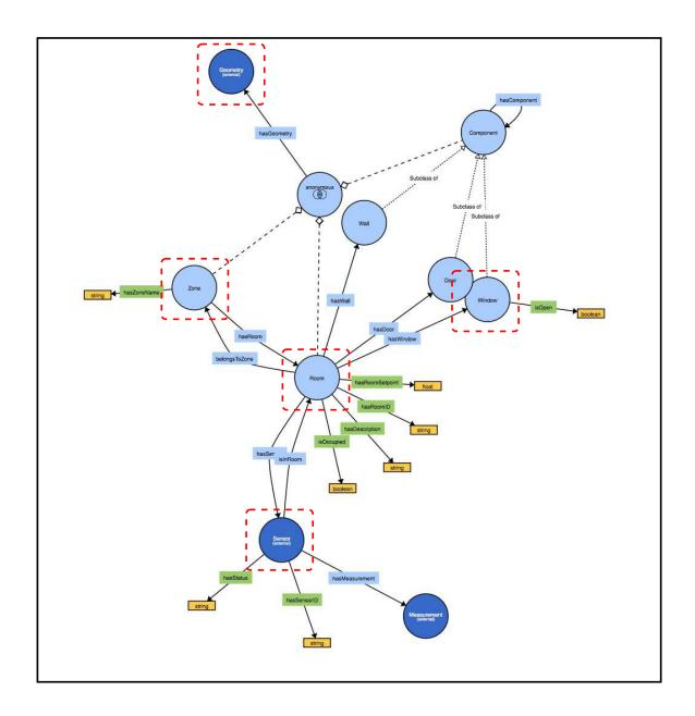
Figure 4.7: Schematic of building ontology classes and properties.
