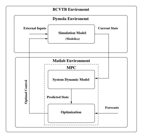
Figure 3.2: Co-simulation framework for integration of model predictive control (MPC) with physical systems simulation with Modelica (Dymola).
