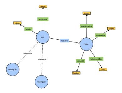
Figure 2.7: Relationship between classes and properties in the component ontology.
