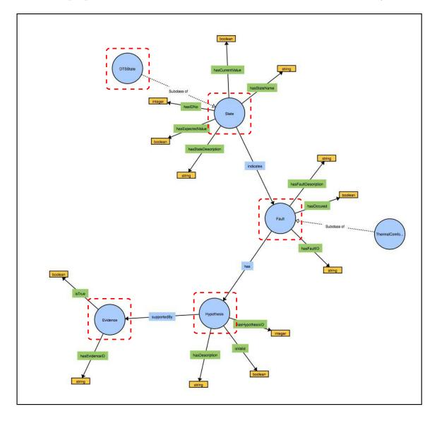
Figure 4.13: Fault detection and diagnostic ontology classes and properties.
