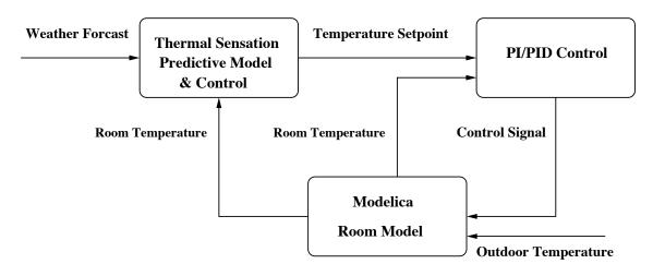
Figure 5.3: Flow diagram for data exchange in BCVTB
