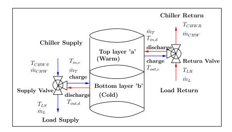
Figure 5.14: Schematic of the thermal energy storage.
