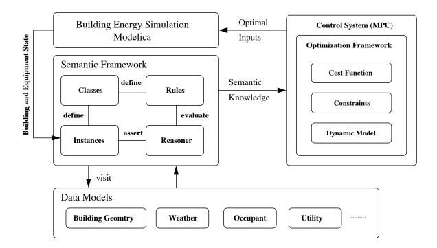
Figure 1.3: Contribution 2: Integration of semantic model with control systems and building energy simulation models.
