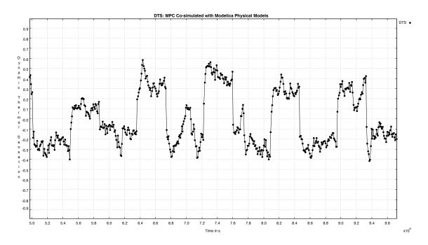
Figure 5.8: Dynamic thermal sensation index versus time (sec) for Control Case 2.
