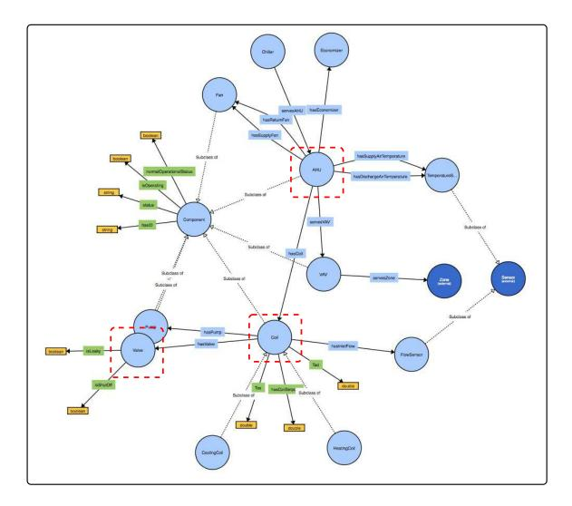
Figure 4.9: Schematic of equipment ontology classes and properties.
