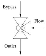
Figure 2.10: Schematic for a three-port valve.
