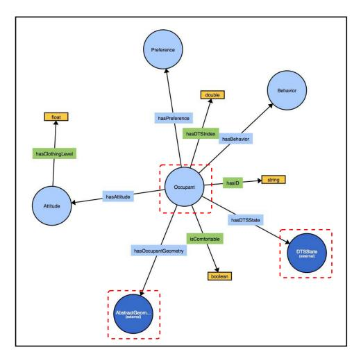
Figure 4.16: Schematic of occupant ontology classes and properties.
