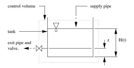
Figure A.6: Front elevation of tank, supply pipe, and exit pipe and valve.
