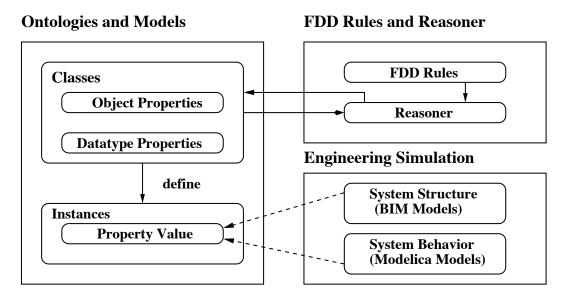
Figure 1.4: Architecture for coupled integrated semantic physical models in building simulations for Fault Detection and Diagnostics (Adapted from Delgoshaei, Austin and Pertzborn [42].
