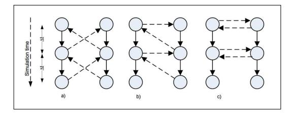
Figure 3.5: Three strategies of data exchange in energy co-simulation: (1) strong coupling of time-dependent states, (2) loose coupling with sequential simulator execution, and (3) loose coupling with parallel simulator execution.
