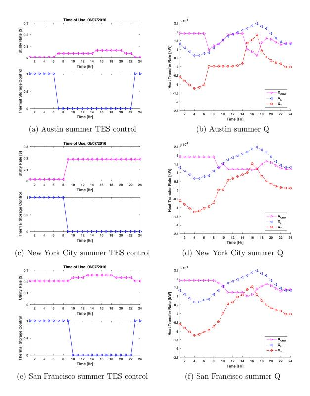
Figure 5.15: Simulation results for Austin, New York City and San Francisco; For TES 1=charge and 0=discharge
