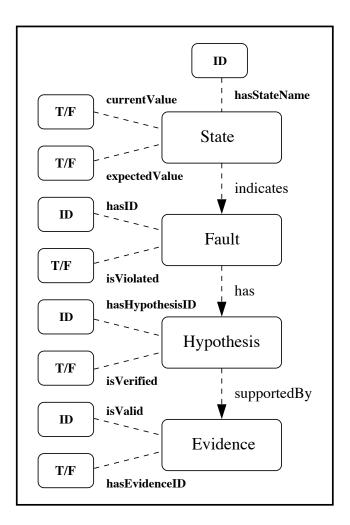
Figure 4.15: Flowchart for identification of faults, and identification and verification of hypotheses and supporting evidence.
