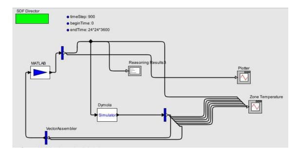
Figure 5.4: BCVTB framework DTS-based MPC and Modelica simulation model.
