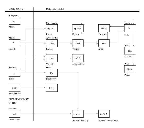
Figure A.1: Primary base and derived units commonly found in engineering mechanics.
