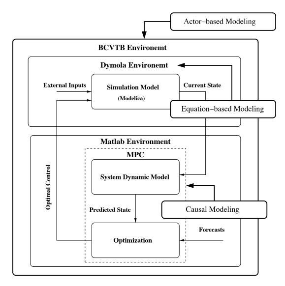
Figure 3.6: Annotated co-simulation framework for integration of model predictive control (MPC) with physical systems simulation with Modelica (Dymola).
