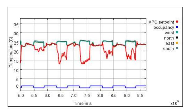
Figure 5.10: Profiles of room occupancy, MPC setpoint, and temperature versus time (sec) for Control Case 2.
