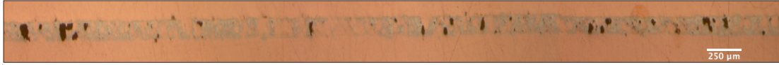
Figure 2-23: Cross-section image of a section of large-area interconnection processed by one-step Cu-Sn TLPS processing under optical microscope
