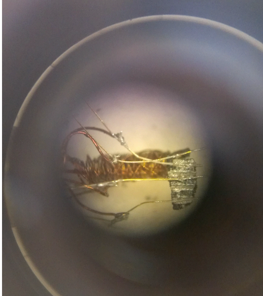
Figure 4.6: The 4-wire resistivity measurement setup for natural bornite sample. The shiny yellow parts are gold thin film fabricated by PVD method; the wires are connected to the gold parts with silver epoxy. The sample is located in the cell which will be filled with pressure medium during the experiment.
