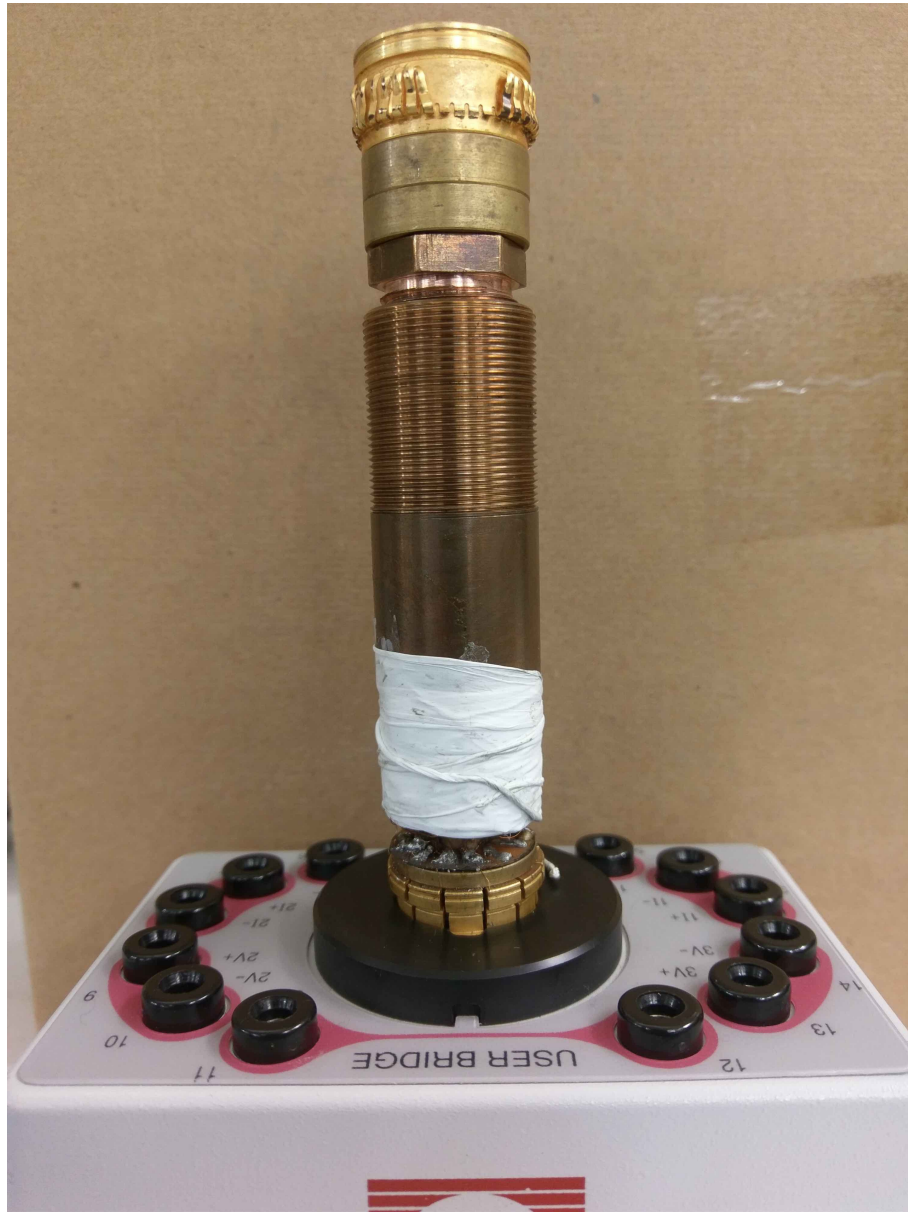
Figure 2.6: Photo of our pressure cell setup. The sample holder was made by me.
