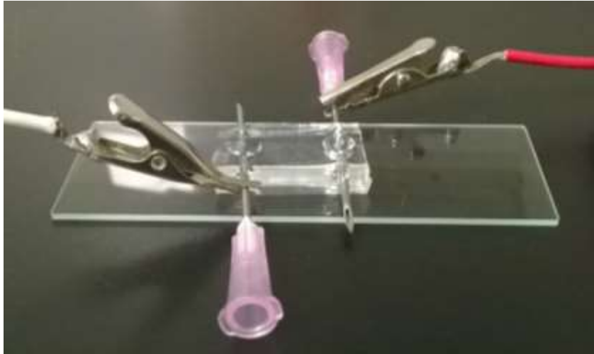
Figure 28. Experimental setup for flow studies in micro-channels.
