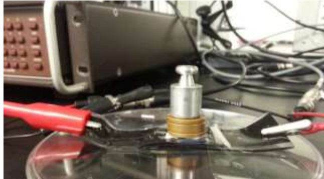
Figure SI 78. Experimental setup for studying the I - V characteristics of the paper-based stacked-layout electroosmotic actuator. The electrodes were connected to a source-measurement unit. The current was recorded as a function of applied voltage, and the influence of applied loads on current was studied.
