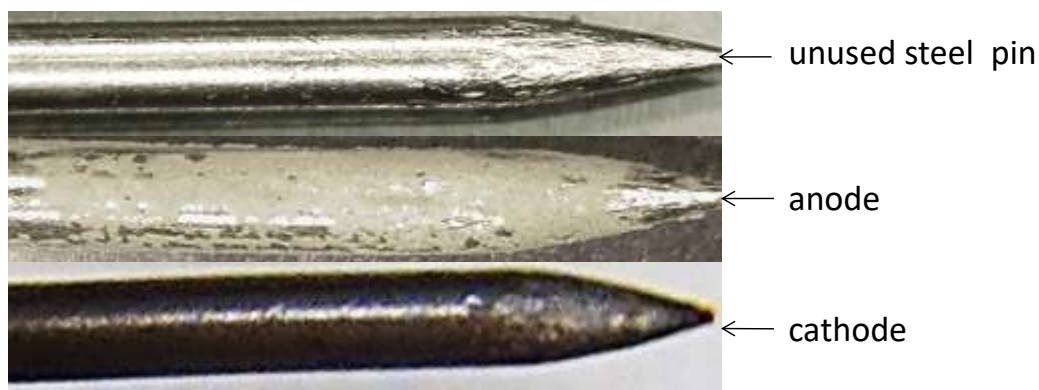
Figure 55. Top: fresh steel pin. Bottom: steel pin used as cathode covered with sticky deposit upon high voltage (3.2 kV) application to degraded PC.
