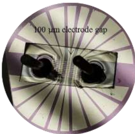
Figure 3. Closely spaced electrodes for low-voltage EOF testing. Device with 5 pairs of electrodes. These electrodes are spaced by a 100 \mu\text{m} gap, and each pair is spaced by 1 mm.
