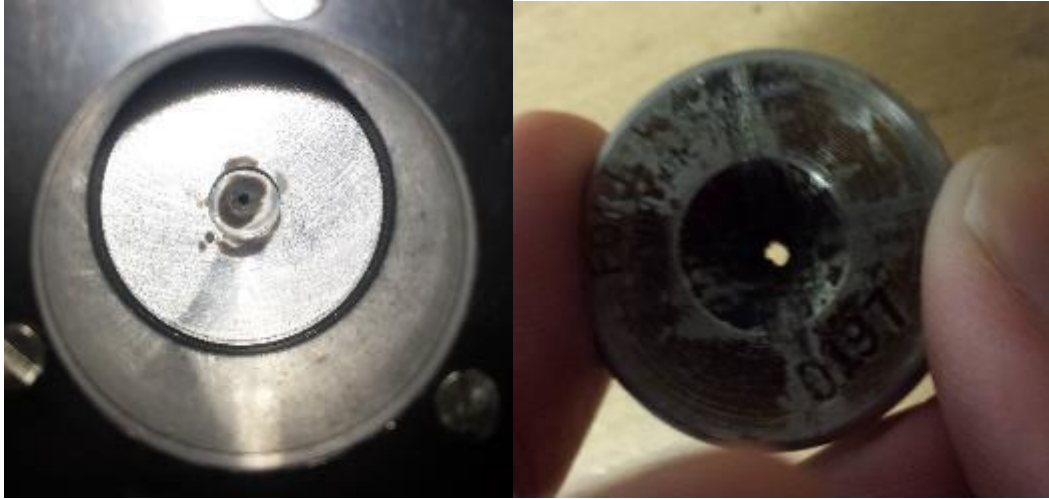
Figure A.10 The aperture in the Nd:YAG regenerative amplifier SFUR(left), and a damaged pinhole used in the Nd:YAG vacuum spatial filter.(right) The SFUR aperture is still a clean, 1mm circle after decades of use. The laser profile is burned around the aperture, showing the extent to which the aperture is overfilled. In contrast, the VSF pinhole is easily damaged by misaligning the high power beam which is focused through it.
