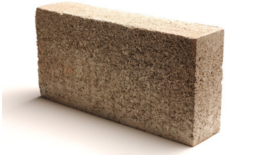
Figure 5 Hempcrete blocks serve as primary thermal and acoustic insulators when they encase a facade (source: Scott Lewis, Flickr)
