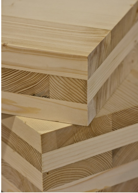
Figure 3 Strong and stable, CLT can be used as walls, roofs, and floors in mid-rise buildings. (source: U.S. Department of Agriculture, Flickr)
