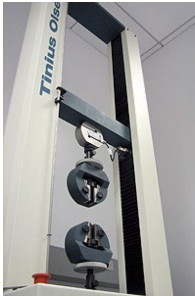
Figure 27. Tinius Olsen H25K-T Benchtop Universal Testing Machine
