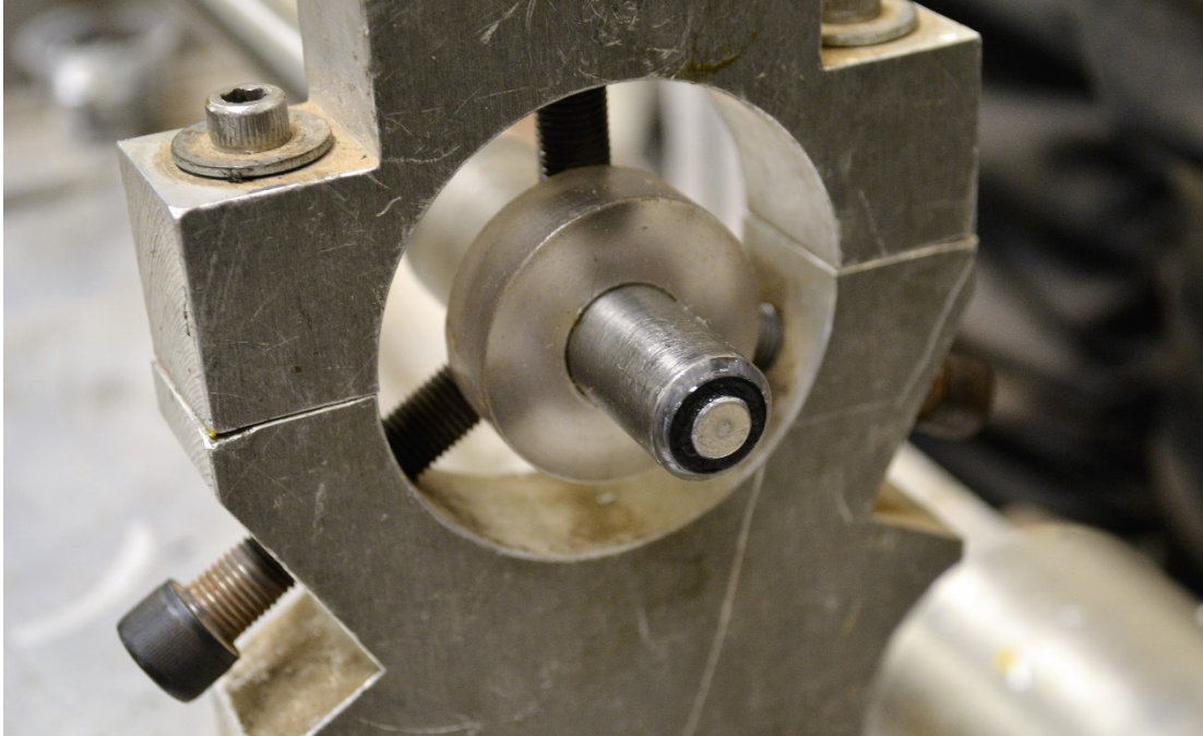
Figure 31. Dual Pulse Shaper Installed on Incident Bar
