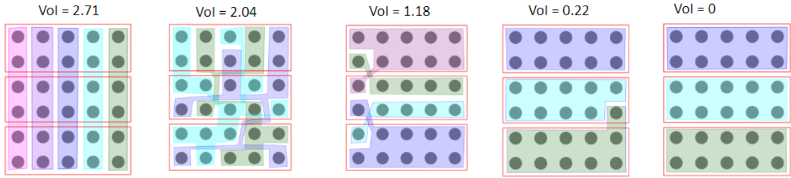
Figure 5.11: Some possible discovered clusterings (colors) compared to the true clusterings (rectangles) and the variation of information (labeled “VoI”) between them
