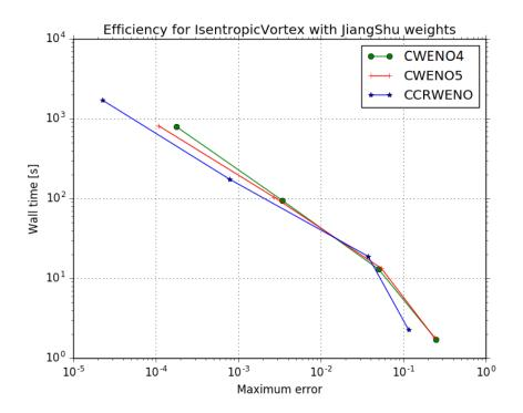
Figure 3.6: CCRWENO outperforms other central schemes in isentropic vortex advection. Markers correspond to the grids in Table 3.4.
