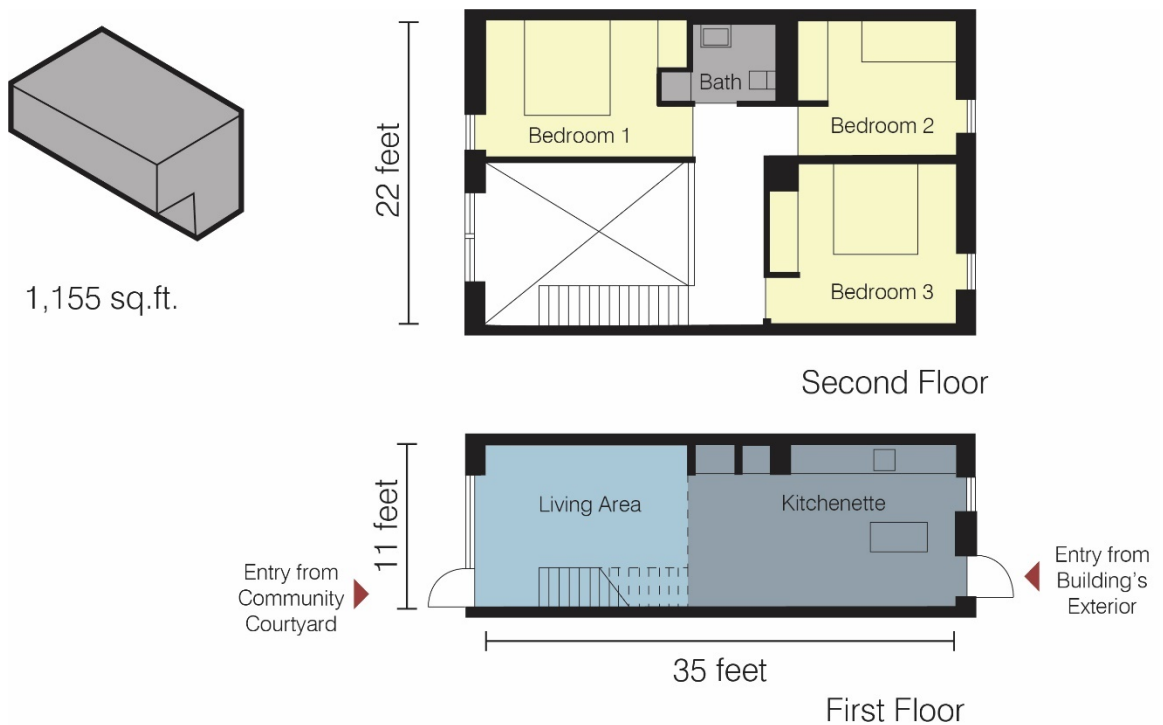
Figure 37: Lange Eng typical three-bedroom unit
