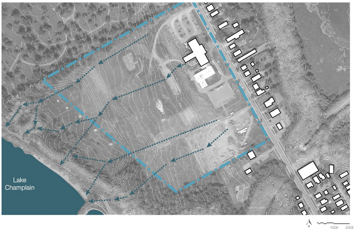
Figure 73: Water flow on site – North Avenue, Burlington
