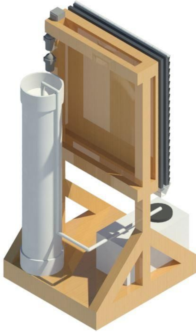
Figure 7. Computer aided design (CAD) drawing rear angle view of prototype biowall construction.
