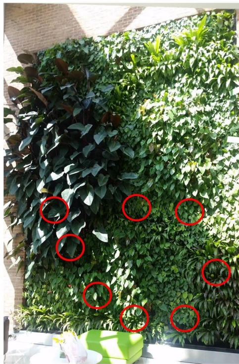
Figure A3. Location of Root Samples on Horace Mann Elementary School Biowall.
