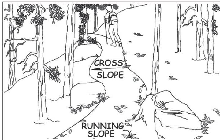
Figure 1. Illustration of running and cross slope ( www.access-board.gov )
