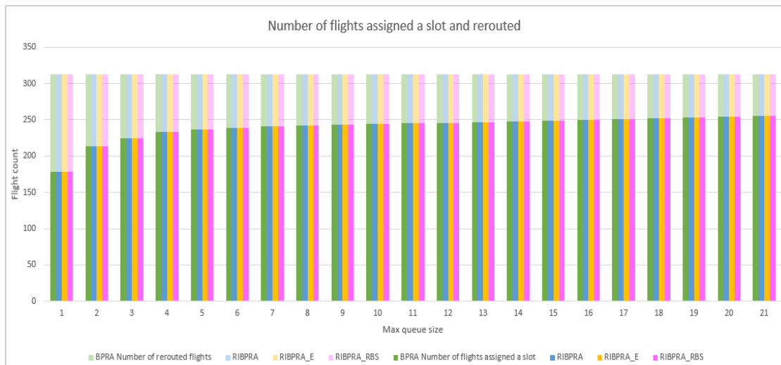
Figure 53: Number of flights assigned a slot and rerouted by max queue size
