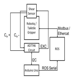
Figure 2.3: Hardware schematic, along with the respective communication protocols
