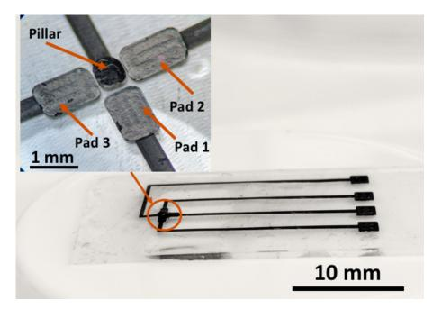
Figure 2.2: Manufactured Sensor
