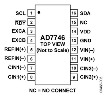
Figure 2.7: Circuit diagram of the AD7746 chip [21]
