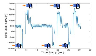
(c) Motor load applied by the isolated finger
