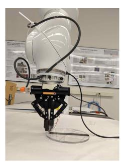
(a) Experimental setup for removing tape
