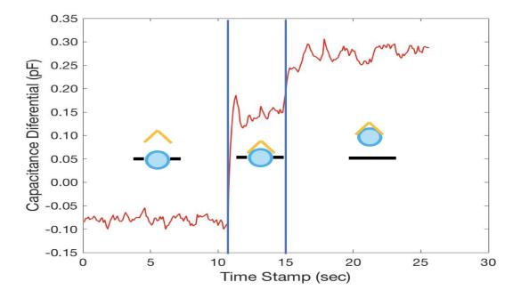
Figure 4.6: Sensor feedback for the grasping and lifting a metallic object
