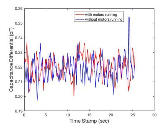
Figure 4.3: Sensor response with no applied load without robot motors running (blue) and with motors running (red)
