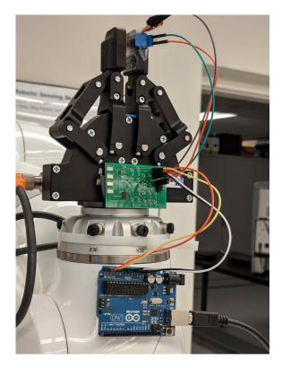
Figure 4.2: Shear sensing system integrated with KUKA iiwa
