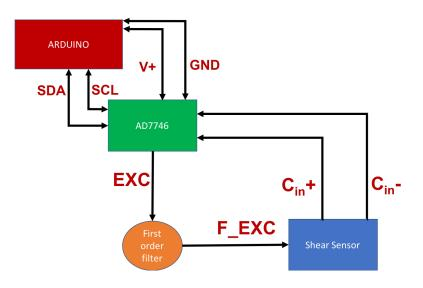
Figure 2.5: Circuit model of the final PCB
