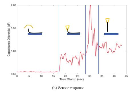
Figure 4.8: Experimental setup and sensor response during tape removal
