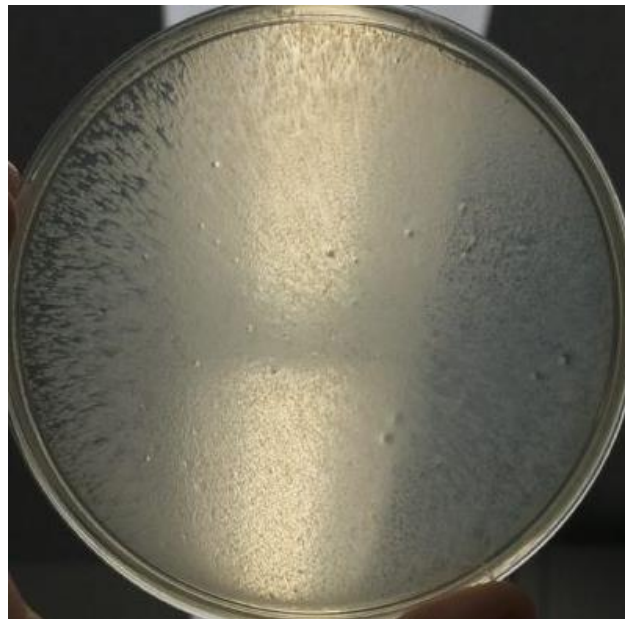
Figure 5: Ascertaining Phage Stock Titer. Titer experiment with semi-solid 1% agar, bacterial concentration of 10^{-10} OD and A511 phage concentration of 10^{-1} of the unknown stock concentration. No visible plaques at such low bacterial concentrations could potentially indicate low phage activity.
