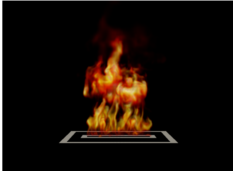
Figure 3.11: Simulated flame structure for the co-flow stabilized, turbulent, buoyant line fire without wind and slope; visualized using volume rendering of temperature.
