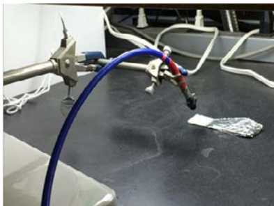
Image 3: Data collection setup with fiber optic spectrometer
