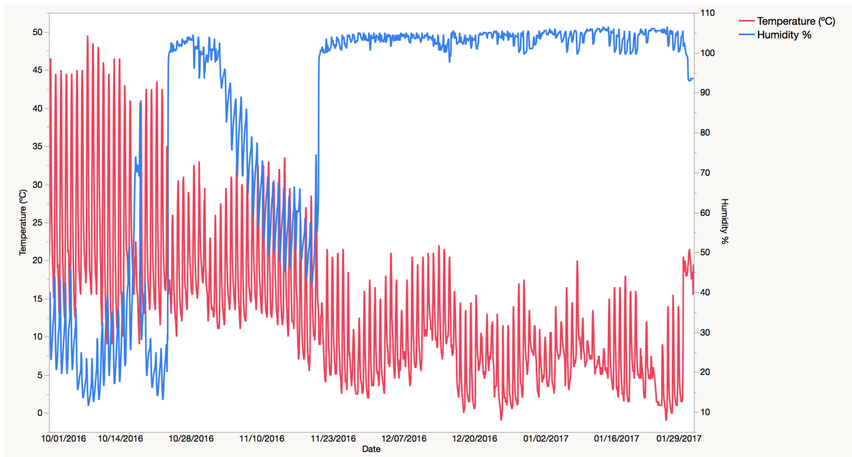
Figure 21. Temperature and humidity data of Data Logger #1 from Swarthout Canyon between October 1, 2016 to January 30, 2017. (Data loggers were removed from soil on January 28.).
