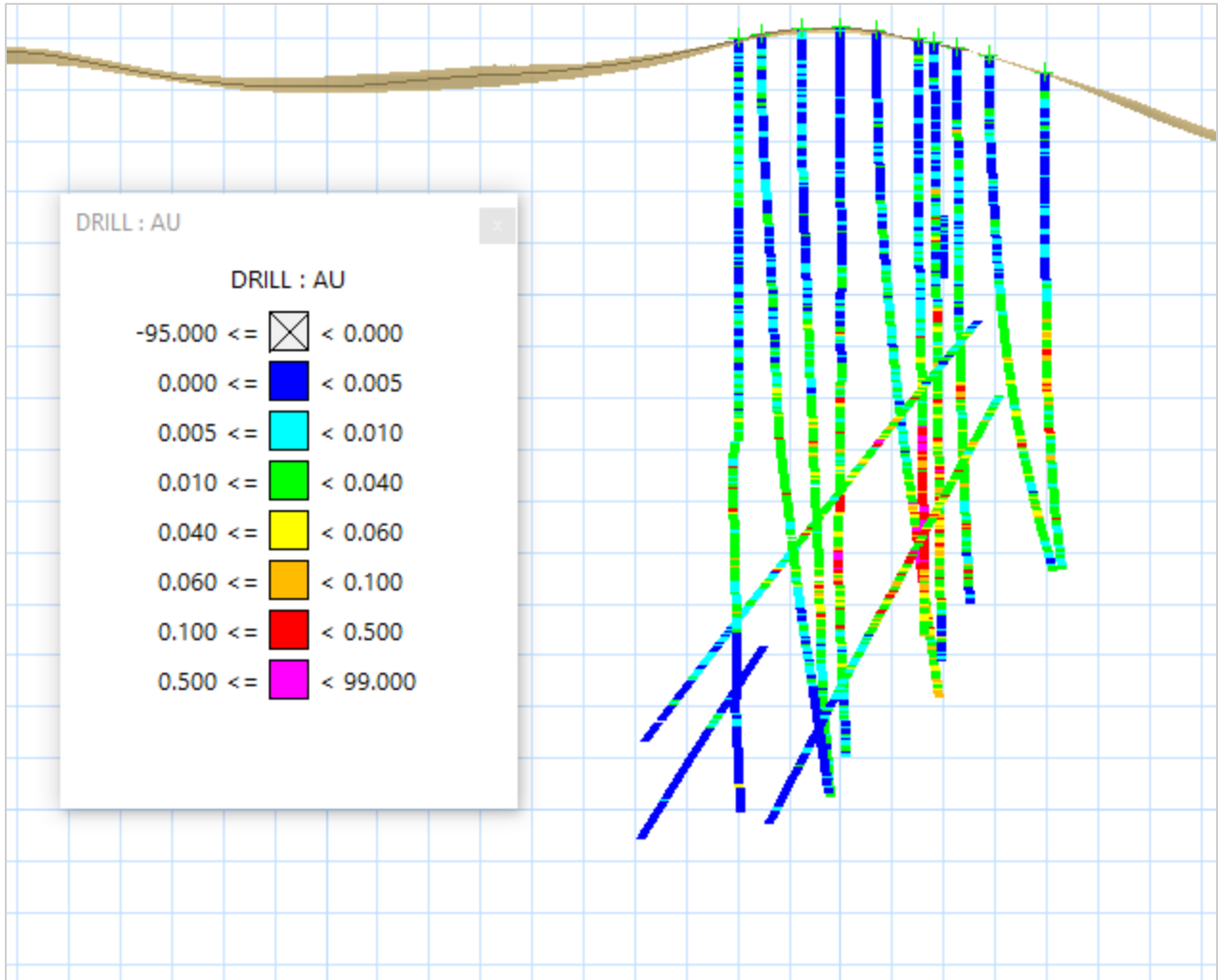
Figure 43: North-South section (left-to-right) of drilling data on the 51,400 ft. easting. Gold grade is displayed along the lengths of the drillholes. Grid spacing is 100 ft.
