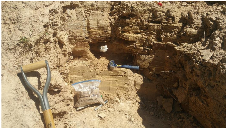
Figure 4: At the Elk Creek Rd section the sample tube is shown in place and capped. A sample bag of surrounding sediment for dose rate measurements was collected from around the tube where the outcrop has been scraped flat
