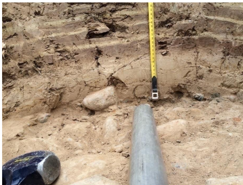
Figure 3: At the Blue Creek Road section, the OSL sample was taken at the contact between overlying sandy silt and underlying sandy-gravel facies. A 25cm long aluminum tube was pounded in the sediment and capped off at the ends.
