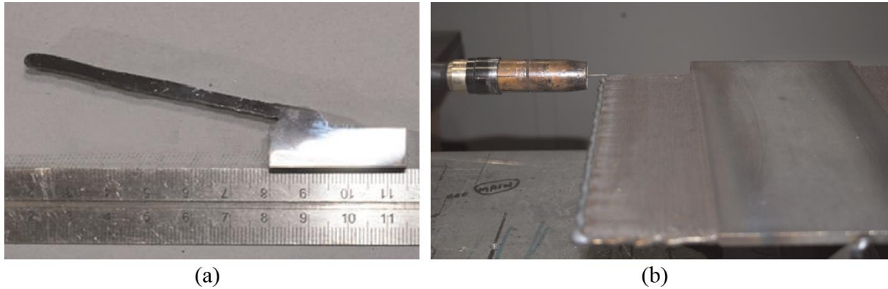
Figure 19: (a) Inclined wall built on flat substrate and (b) horizontal wall built on substrate edge using the inclined torch GMAW WAAM technique. Adapted from [31].
