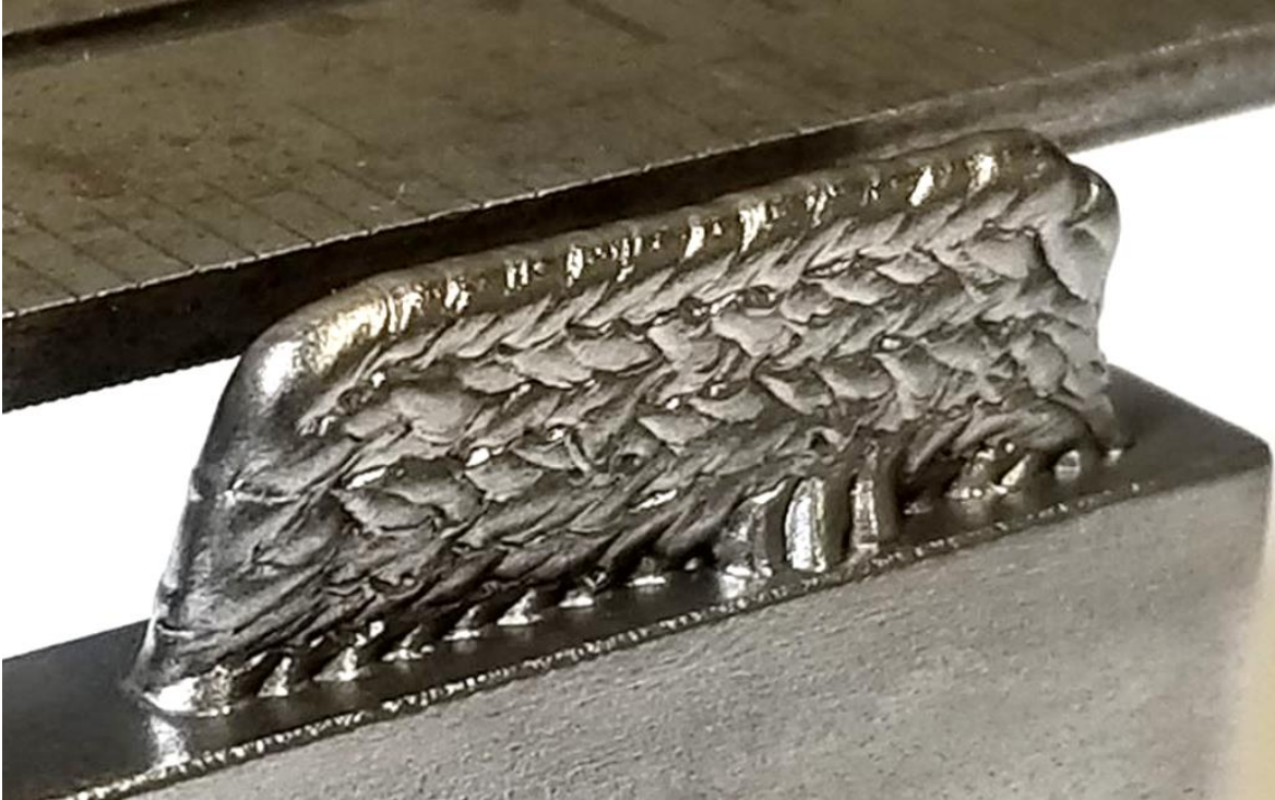
Figure 116: HFS4 specimen manufactured using SiDD with high frequency arc starting using ER70S-3 wire and 98% Ar, 2% O 2 shielding gas.
