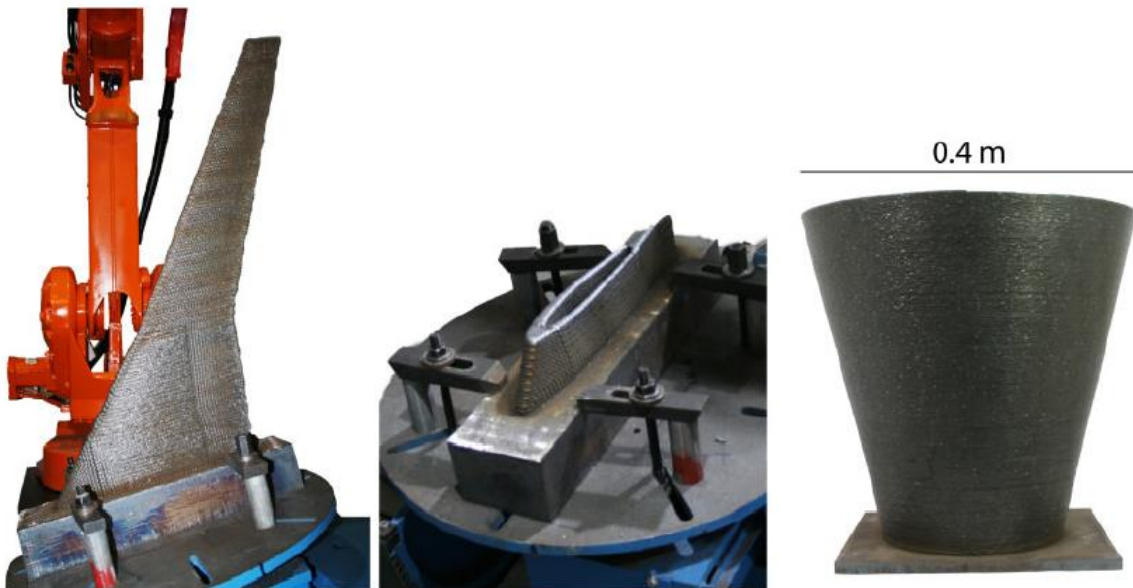
Figure 26: Components manufacture with WAAM using CMT [8].
