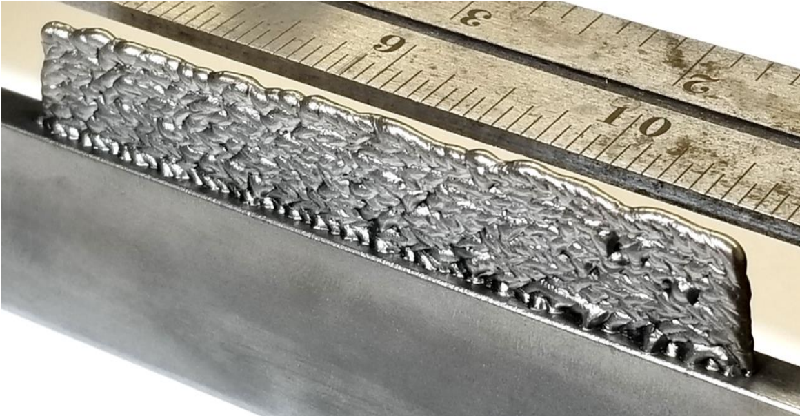
Figure 111: HFS1 specimen manufactured using SiDD with high frequency arc starting using ER70S-3 wire and 98% Ar, 2% O 2 shielding gas.
