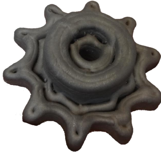
Figure 14: Simple component made with the open-source metal 3-D printing system. Adapted from [23].
