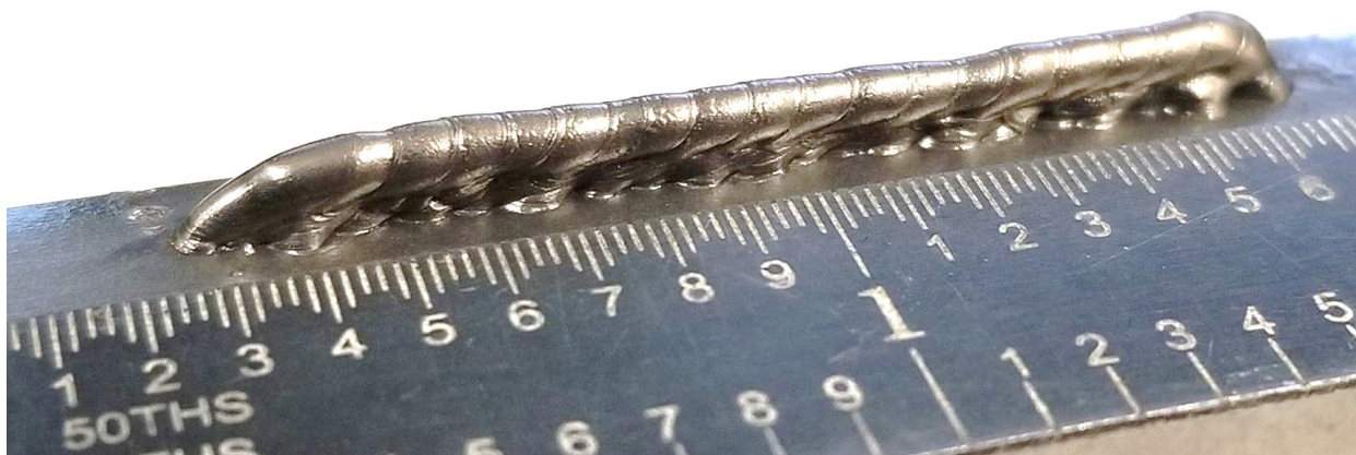
Figure 99: Two layers deposited using SiDD with PAW pilot arc starts. Both layers were deposited one drop at a time from right to left using ER70S-6 wire and 98% Ar, 2% O 2 shielding gas.
