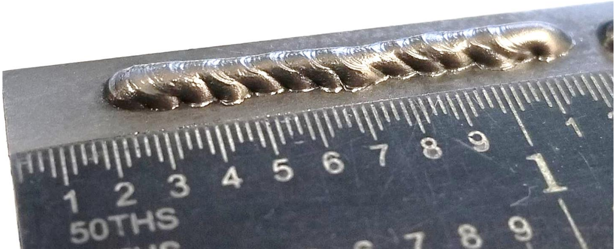
Figure 98: Weld bead deposited using SiDD with PAW pilot arc starts. The weld bead was made by depositing one drop at a time from left to right using ER70S-6 wire and 98% Ar, 2% O 2 shielding gas.
