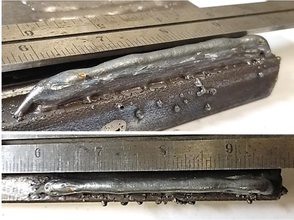
Figure 87: Wall built with continuous weld beads using ODPP pulsing parameters with ER70S-3 wire and 98% Ar, 2% O 2 shielding gas.
