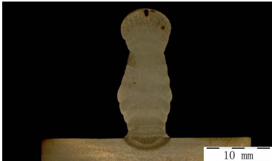
Figure 17: Weld bead width control depositing various bead widths on each layer [29].
