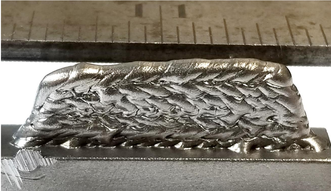
Figure 114: HFS2 specimen manufactured using SiDD with high frequency arc starting using ER70S-3 wire and 98% Ar, 2% O 2 shielding gas.
