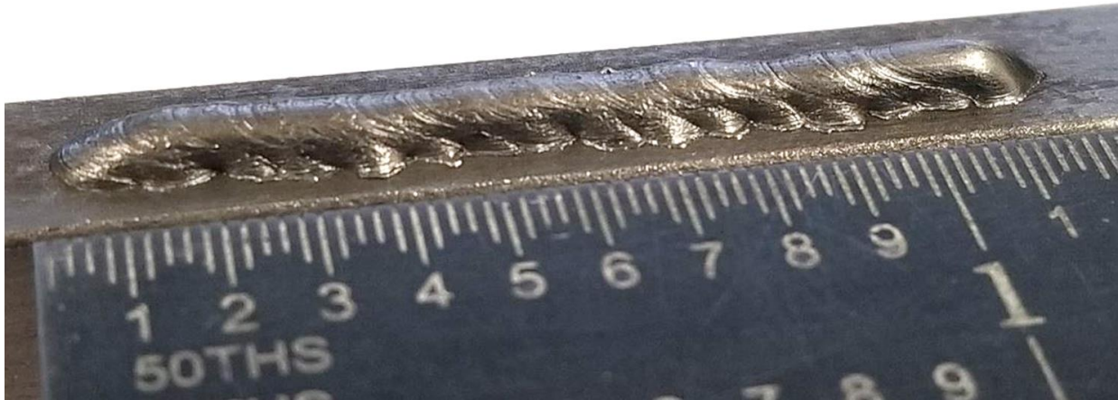
Figure 103: Weld bead made using automated SiDD with hybrid arc starting. The weld bead was made by depositing one drop at a time from left to right using ER70S-3 wire and 98% Ar, 2% O 2 shielding gas.
