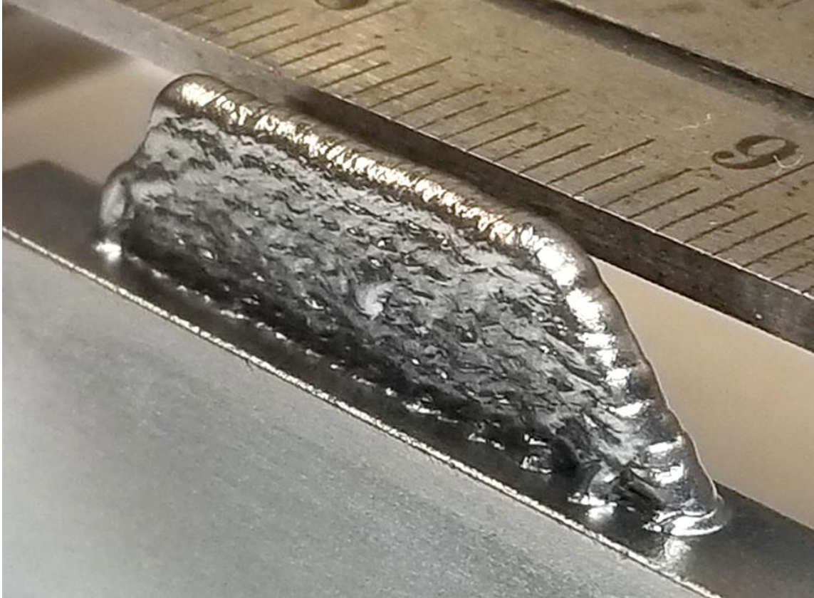
Figure 117: HS1 specimen manufactured using SiDD with laser hybrid arc starting using ER70S-3 wire and 98% Ar, 2% O 2 shielding gas.
