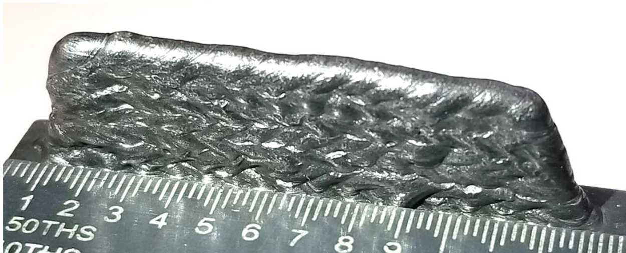
Figure 115: HFS3 specimen manufactured using SiDD with high frequency arc starting using ER70S-3 wire and 98% Ar, 2% O 2 shielding gas.
