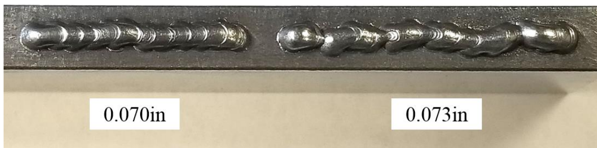
Figure 113: Drop spacing comparison. A drop spacing of 0.070in produced a more uniform weld bead compared to the drop spacing of 0.073in.
