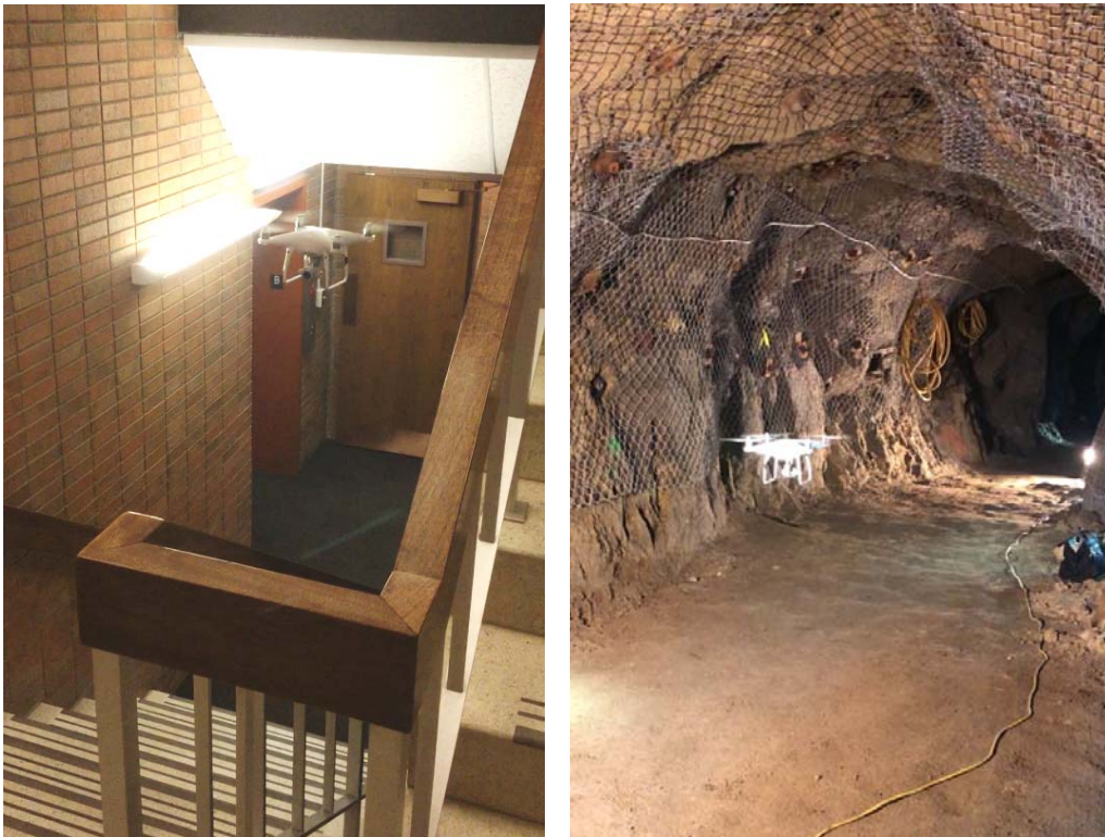
Figure 8. Photos of ( Left ) an out of LOS flight with P4P in the basement of the MG building and ( Right ) the P4P flight in UMEC where Tripod Mode was tested and terrestrial lighting was used to light the rock face.
