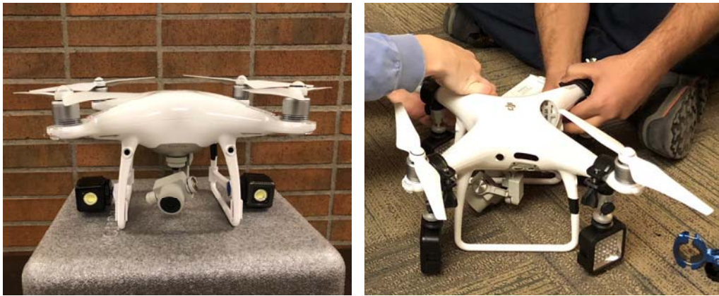
Figure 25. Left: Lume Cube lights attached to P4P for testing, Right: Firehouse Technology lights used for testing on-board the P4P.
