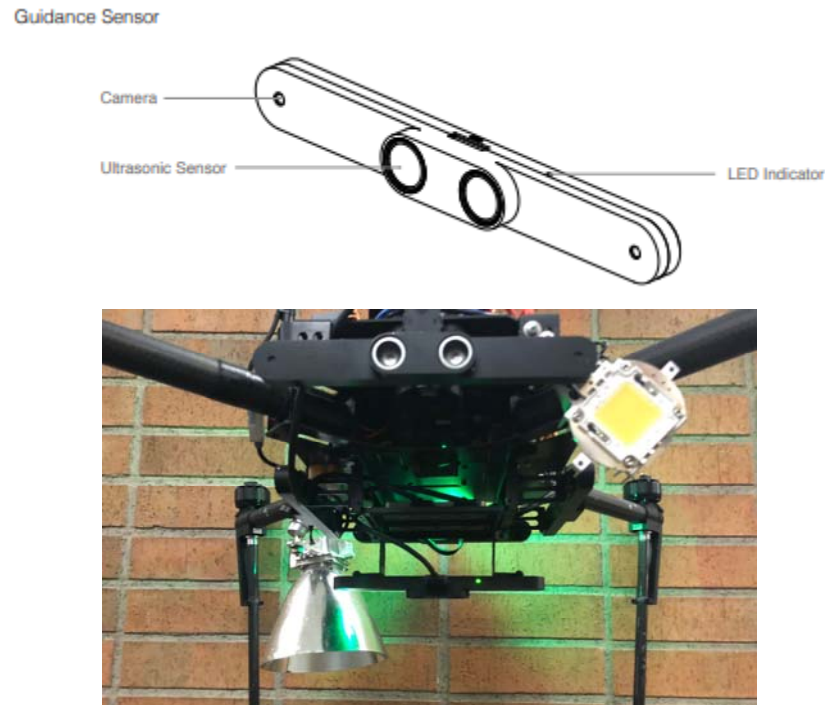
Figure 3. (Top) An example of one of the five sensors that use LED indicators to confirm if the Guidance system is being used for detecting obstacles through the DJI Guidance cameras and ultrasonic sensors (DJI GUIDANCE User Manual, 2015) and (Bottom) the DJI Guidance mounted to the bottom of the M100 UAV.
