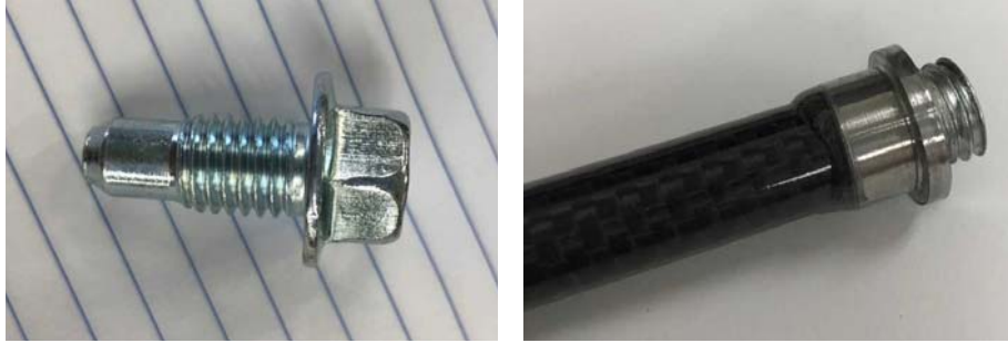
Figure 26. Before ( left ) and after ( right ) photos of one of the automobile drain plugs that was machined to create customized UAV leg connectors for the M100.
