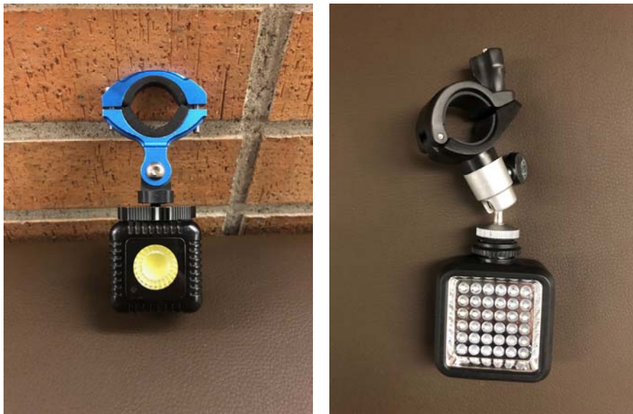
Figure 6. Left: Lume Cube and connector used for attaching Lume Cubes to M100, Right: Firehouse Technology Light and connector used for attaching the Firehouse Lights to the M100.
