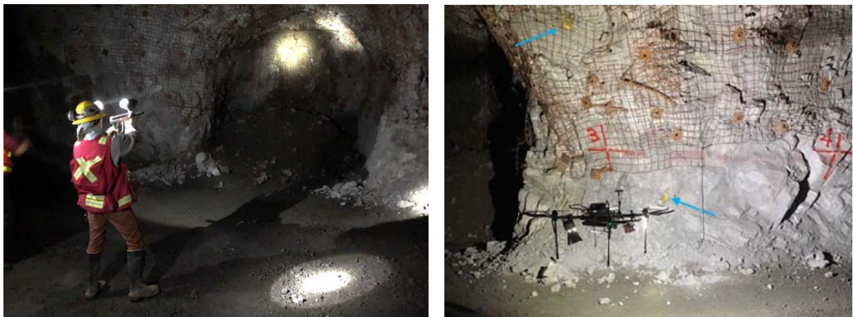
Figure 11. (Left) UAV team member shooting paintballs onto ribs for creating control points and, (Right) Control points created on the ribs in yellow (blue arrows are pointing to paintball marks). For scale the height of the paintball gun operator in the image to the left is 1.7 m (5ft. 7in.) tall. In the photo to the right, the wire mesh has 25 mm (4 in.) spacing and the UAV (with the propeller guards) measures about 1.2 m (4 ft.) diagonally.
