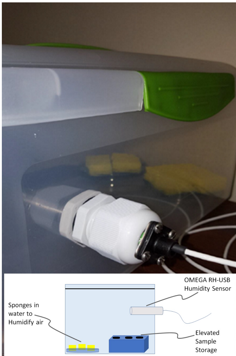
Figure 22. Custom humidity ageing chamber which enabled the rapid ageing of HP composites in high humidity conditions. Humidity and temperature ( RH\ 90.3\% \pm 4.9\% at 20.24\ ^\circ C \pm 1.26\ ^\circ C ) monitored continuously using an Omega RH-USB sensor. Inset, a schematic of the components of the humidity chamber.
