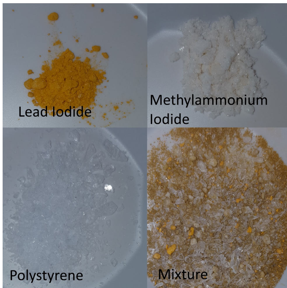
Figure 57. HP precursors (top), polystyrene feedstock (bottom, left), and the simple mixture (bottom, right) of all three into the melt ES feedstock material. From Murphy et al. [100]
