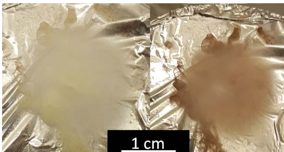
Figure 66. An electrospun fiber mat immediately after ES (left) and after 5 min in ambient condition (right). The color change of the fiber mat is indicative of the HP reaction occurring as residual solvent evaporates in the fibers, from Murphy et al. [103].
