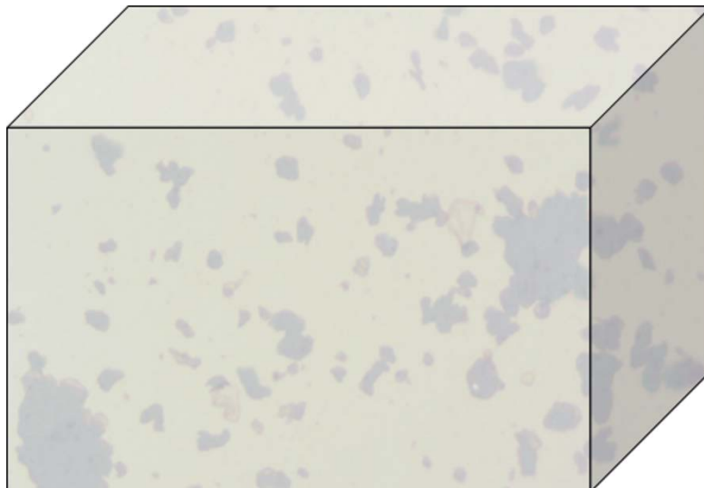
Figure 7. Diagram of a typical composite with a continuous matrix phase and a dispersed filler phase. Agglomerations of the filler phase can occur when the polymer melt/solution does not wet the filler particles, whereas a well-dispersed composite is the result of a high degree of wetting of the filler phase.
