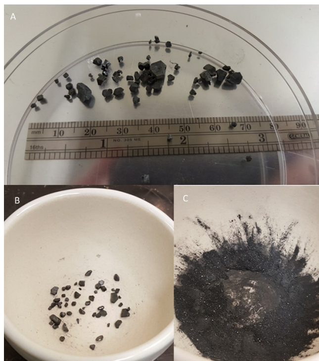
Figure 40. Average quantity of \text{CH}_3\text{NH}_3\text{PbI}_3 single crystals produced from a 10 mL batch of solvent (A). The mechanical milling via mortar and pestle of the single crystals into a powder for further processing (B & C).
