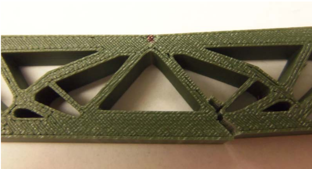
Figure 37: MATLAB penalized beam, P1 fracture location
