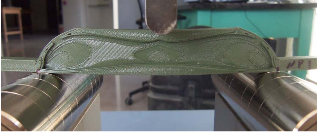
Figure 39: MATLAB non-penalized beam, NP1 setup in three point loading
