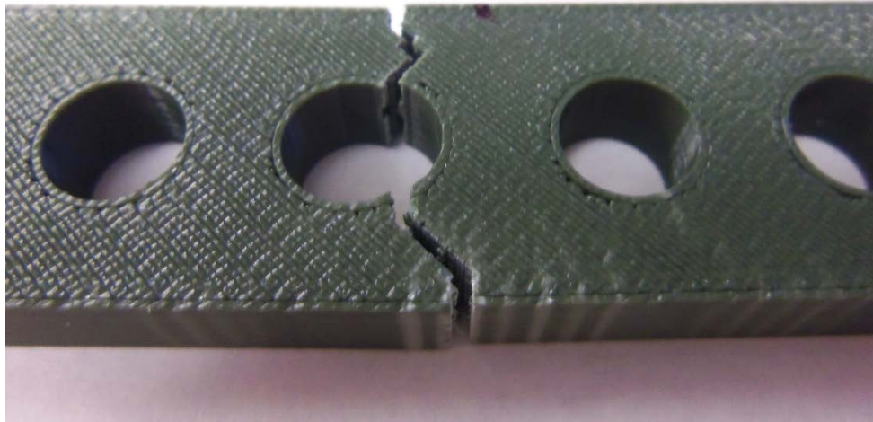
Figure 31: Fracture of beam H1
