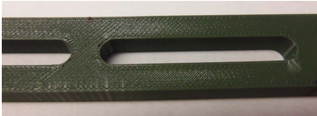
Figure 34: Yielding locations in slotted beam, S1
