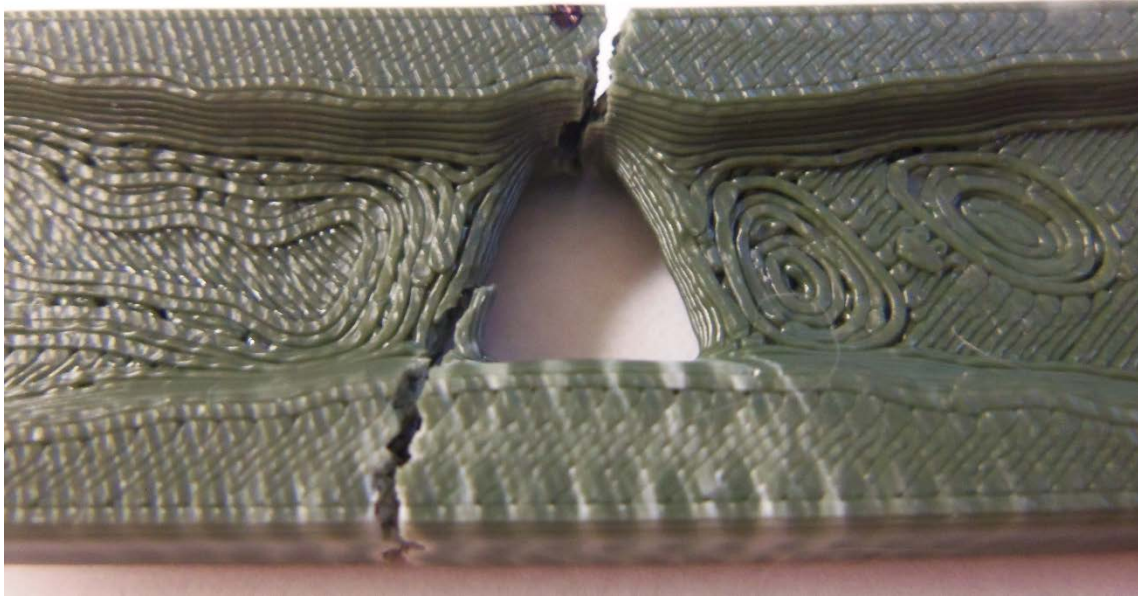
Figure 44: ParetoCloud beam, fracture location and propagation path
