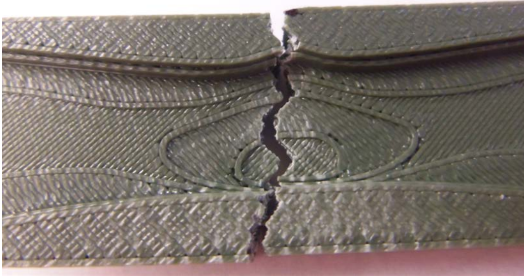
Figure 40: MATLAB non-penalized beam, NP1 fracture location
