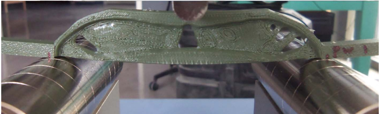
Figure 43: ParetoCloud beam, PW1 in three point loading test
