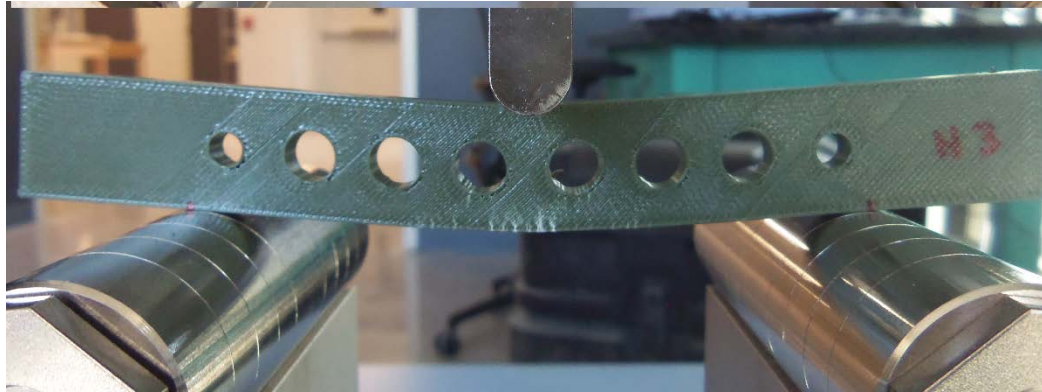
Figure 30: Beam with lightening holes in the three-point loading test
