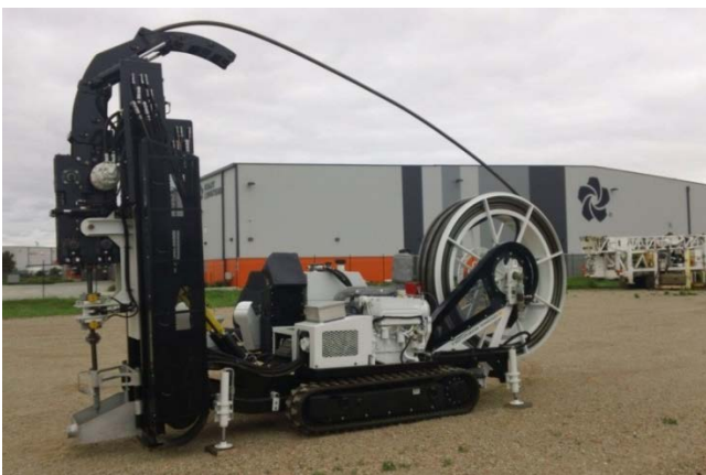
Figure 9: The prototype developed by the DET CRC. This drill rig utilizes the coil tube technology for mineral exploration (Probert, 2013).
