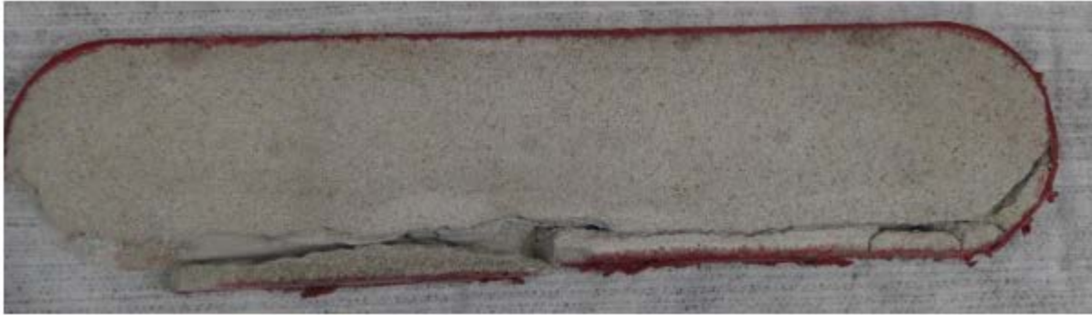
Figure 1: Sandstone Platen Shear Failure Blair (2015)
