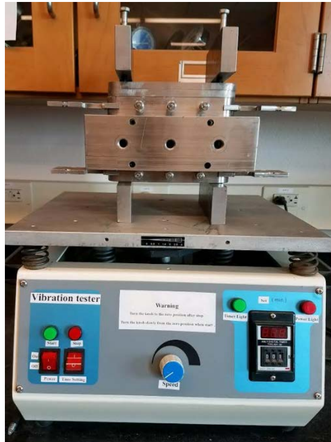
Figure 12: Loaded Hooke Cell with Clamps on VTM
