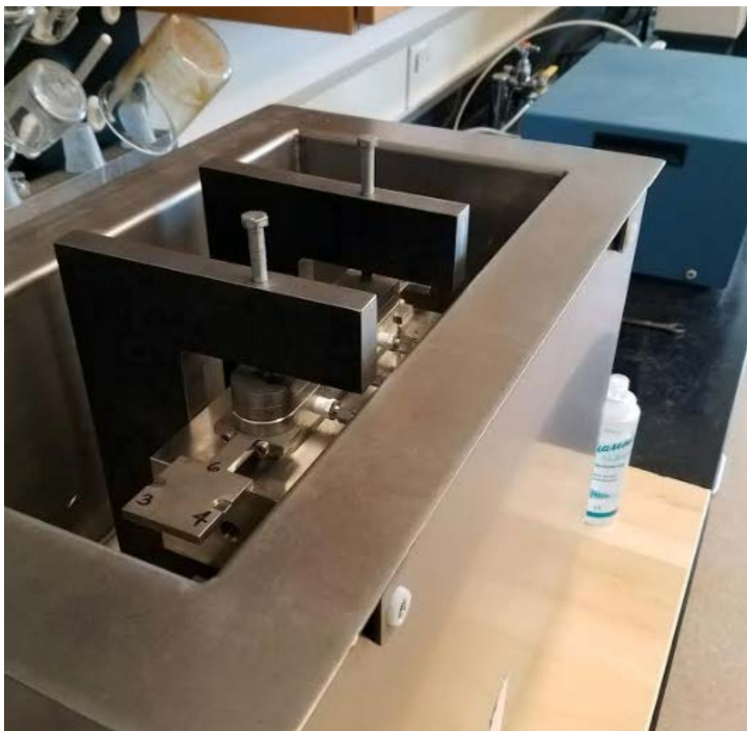
Figure 14: Loaded Hooke Cell with Clamps in SRV Vessel
