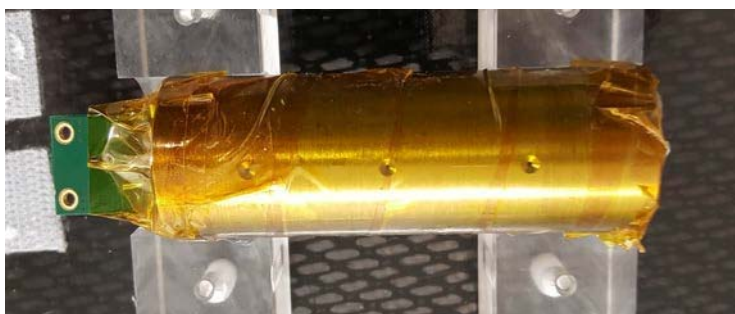
Figure 1. The BrachyView probe covered in a 700 \mu\text{m} kapton tape, in order to ensure no liquid penetration during acquisition.
