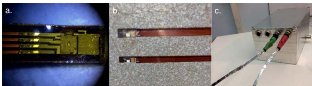
Figure 1. (1a) Diode bonds and silicon sensitive chip ( 1.5 \times 1.5 \times 0.038 \text{ mm}^3 as viewed under a microscope). The bonds were covered for protection (b), and the complete diode assembly is used in conjunction with the in-house produced reader (c).
