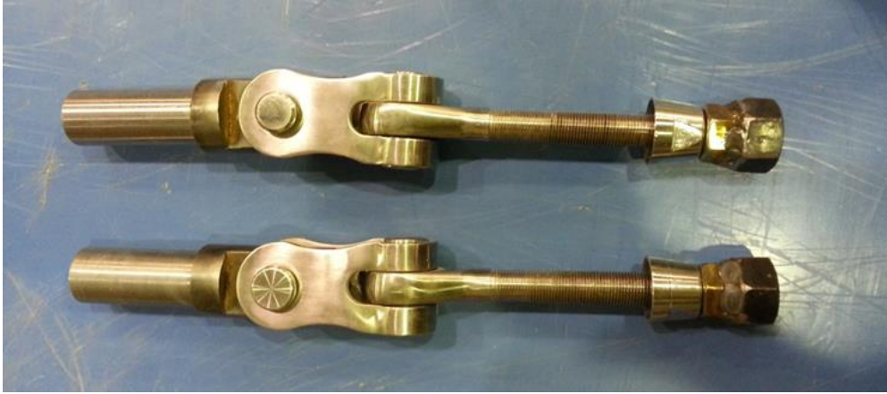
Figure 2.4: Universal joints designed for direct tensile testing of SCC specimen
