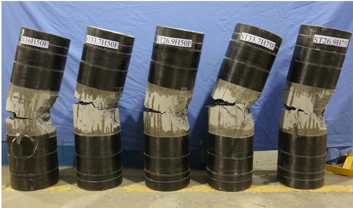
Figure 6.16: Failure modes of specimens tested under flexural loading
