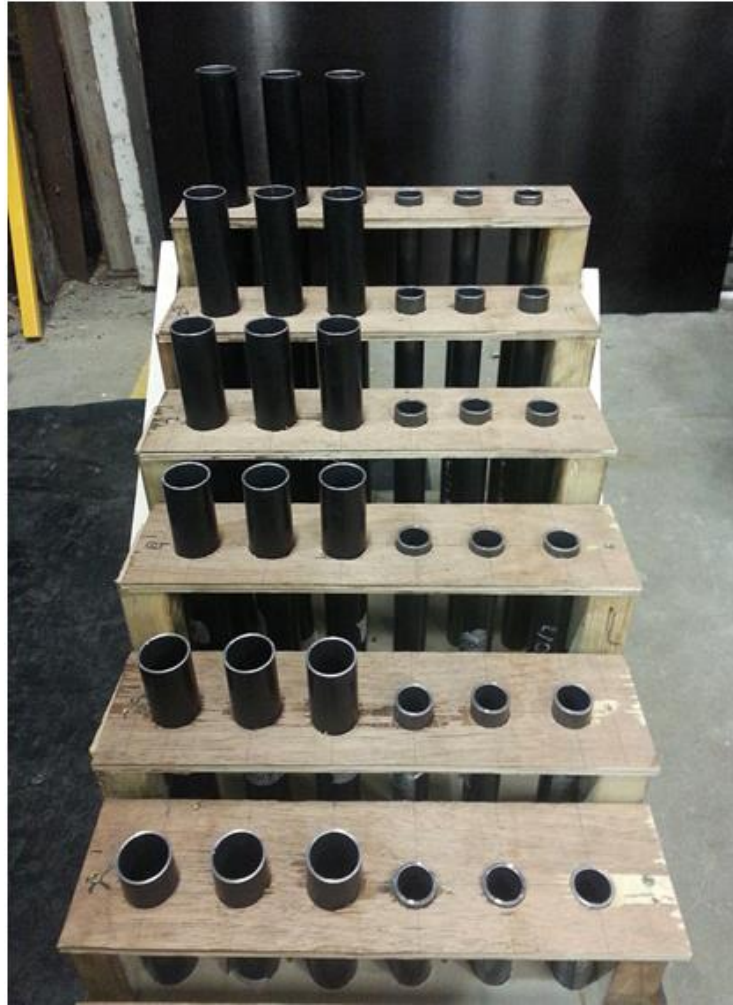
Figure 5.1: Construction of formwork
