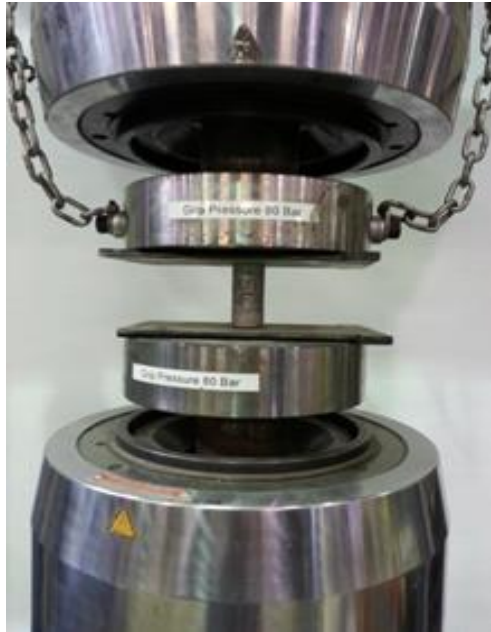
Figure 4.2: Testing of specimen under axial compression
