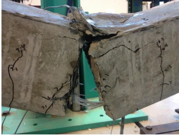
Figure 6. Rupture of GFRP reinforcement bars (Beam 66-0.5-4)
