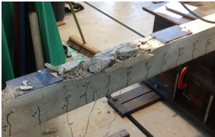
Figure 8. Flexural response with crushing of concrete cover (47-1.0-4)
