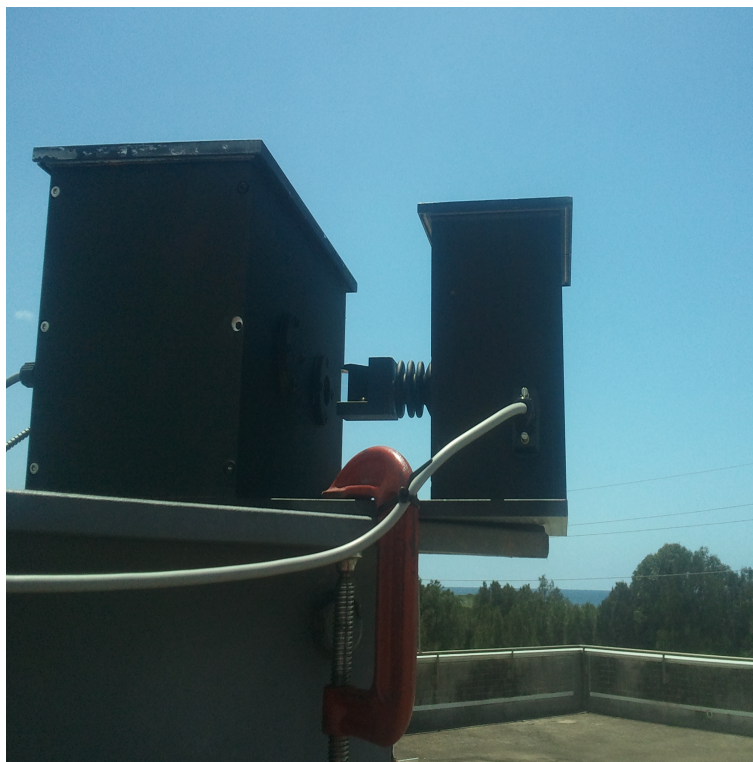
Fig. 2.6: Photo of MAX-DOAS taken during the campaign. The instrument was positioned towards the open ocean looking towards the north-east (68°).
