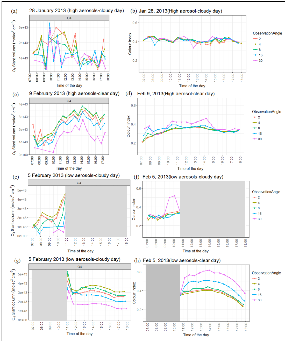
Fig. 5.9: Time series of O_4 DSCD observations and colour Index at five observation angles ( 2^\circ , 4^\circ , 8^\circ , 16^\circ and 30^\circ ) on the 28^{th} January, 2013, 9^{th} February, 2013 and 5^{th} February, 2013. The rectangular shaded areas on the 5^{th} February, 2013 highlight two situations chosen :Fig. (e) and (f) are observations for “low aerosol loading and cloudy day”, Fig. (g) and (h) are observations for “low aerosol loading and clear day”. Measurement data from 7:00 to 17:00 were used in these plots.
