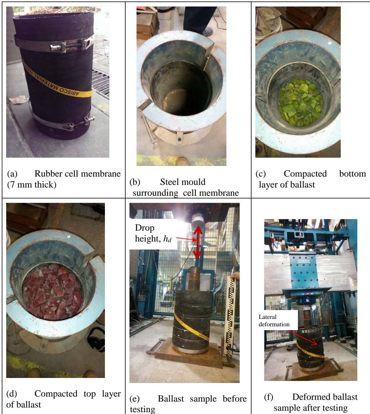
629 Figure 4. Sample preparation: (a) cell membrane; (b) steel mould, (c) ballast at bottom layer; (c) 630 ballast on top layer; (d) ballast specimen; and (f) deformed shape of ballast specimen
