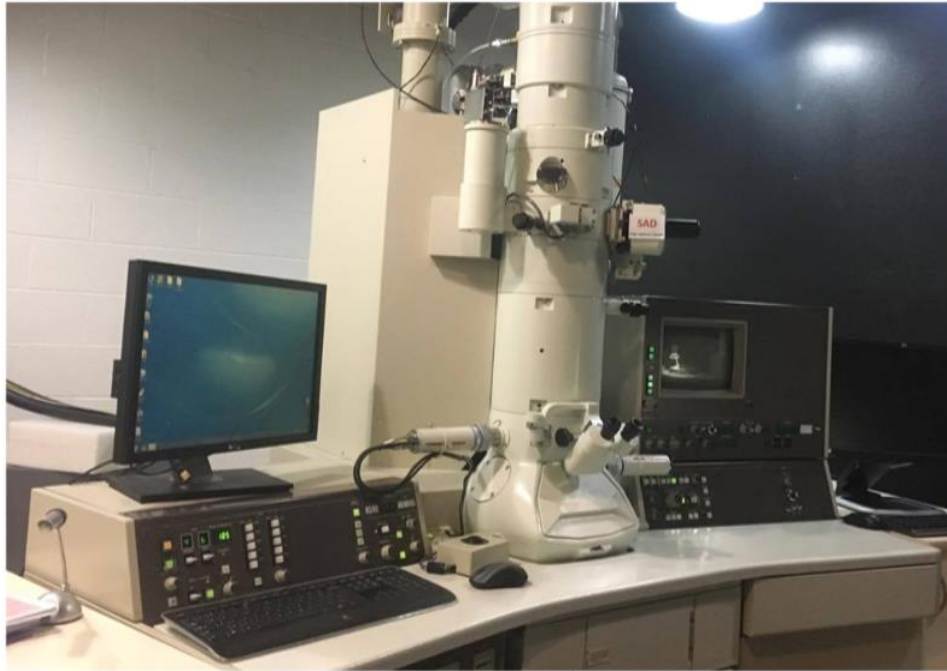
Figure 2.7: TEM model JEOL JEM-2010 used.
