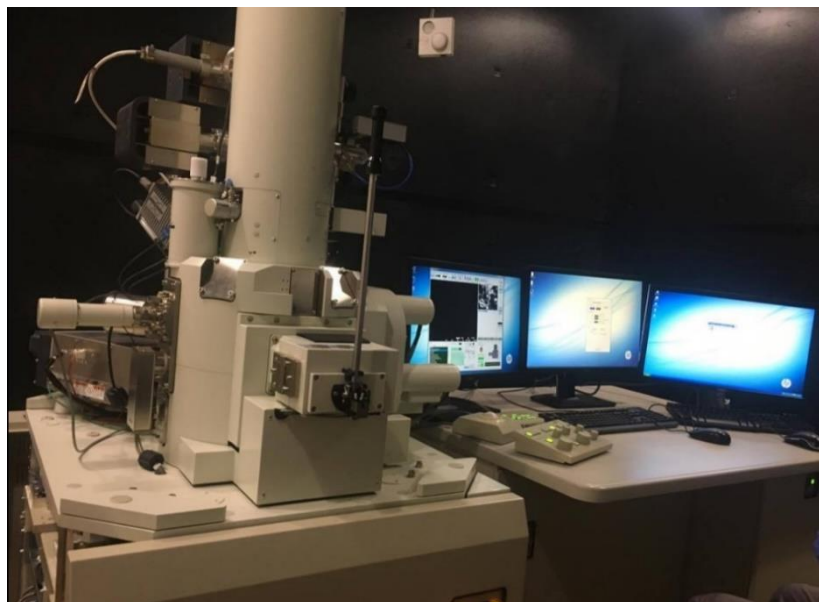
Figure 2.6: Jeol 7500 field emission scanned electron microscope utilized in the study.
