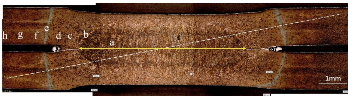
Figure 5. Low-magnification optical microstructure of a whole spot welding joint obtained at AC-6, with a peak current of 12 kA, frequency of 110 Hz, and welding time of 35 cycles.
