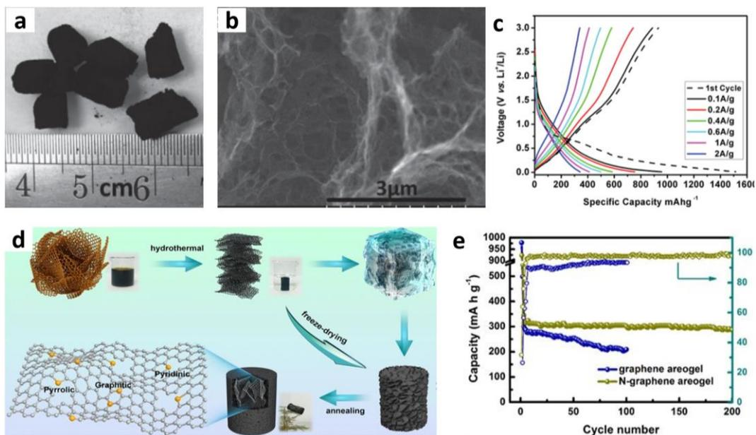
**Figure 4.** (a) Photograph and (b) SEM image of the 3D graphene foam, (c) Discharge-charge curves at different current densities of 3D graphene as anode for LIBs;<sup>[75]</sup> Reproduced with permission, Copyright 2015, John Wiley and Sons. (d) Schematic illustration of the synthesis approach and the application of 3D rGO aerogel, (e) Cycling performance and corresponding Coulombic efficiency of the 3D rGO aerogel.<sup>[76]</sup> Reproduced with permission, Copyright 2017, Springer Nature.
