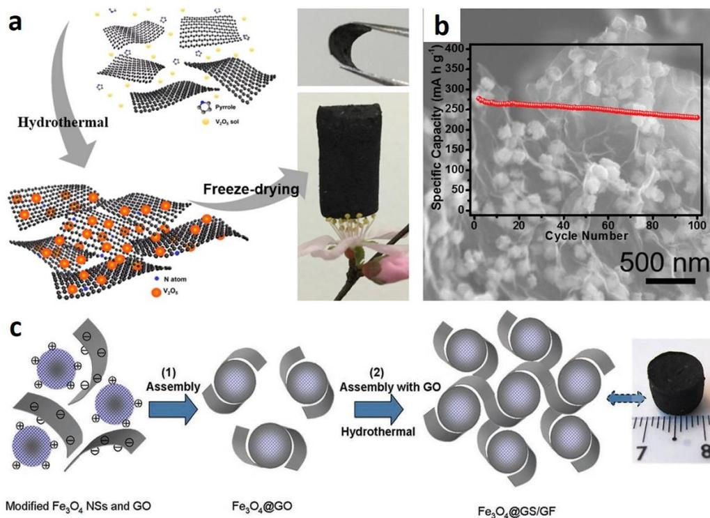
**Figure 6.** (a) Schematic illustration of the synthesis of  $V_2O_5$ @graphene aerogel, and corresponding photographs, (b) SEM image of  $V_2O_5$ @graphene aerogel and its cycling performance (inset),<sup>[91]</sup> Reproduced with permission, Copyright 2018, Elsevier. (c) Fabrication process and photograph of  $Fe_3O_4$ @GS/GF.<sup>[93]</sup> Reproduced with permission, Copyright 2018, Elsevier.
