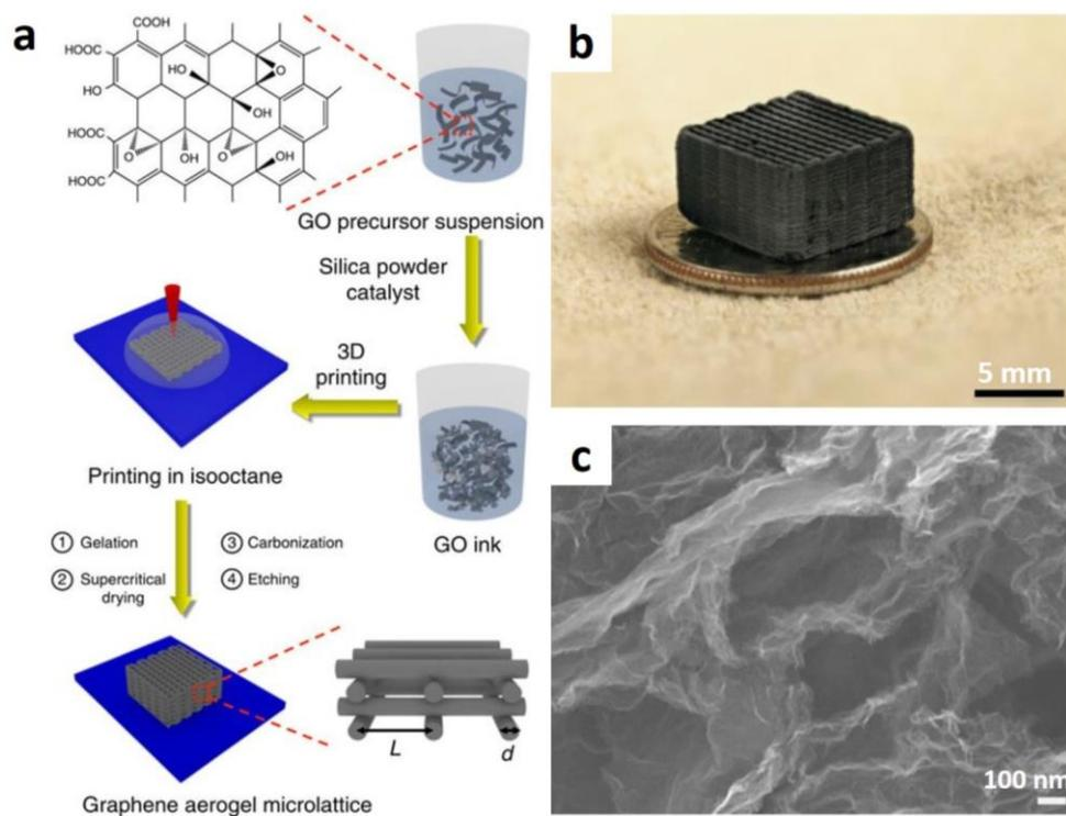
**Figure 2.** (a) Synthesis process for a 3D-printed graphene aerogel microlattice; (b) Digital photograph and (c) SEM image of the 3D-printed graphene aerogel microlattice.<sup>[64]</sup> Reproduced with permission, Copyright 2015, Springer Nature.
