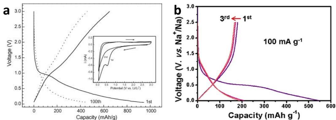
**Figure 3.** (a) Discharge-charge curves of the first two cycles and corresponding CV curves (inset) of graphene as anode for LIBs;<sup>[73]</sup> Reproduced with permission, Copyright 2009, Elsevier. (b) Discharge-charge curves of the first three cycle of graphene as anode for SIBs.<sup>[74]</sup> Reproduced with permission, Copyright 2016, Elsevier.
