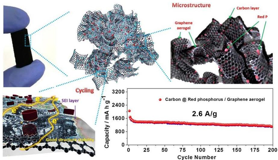
**Figure 7.** Photograph of the C@P/GA, and schematic illustration of its structural advantages, as well as its Na<sup>+</sup> storage performance.<sup>[103]</sup> Reproduced with permission, Copyright 2016, John Wiley and Sons.
