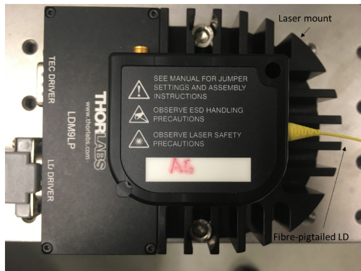
Figure 3.18. Laser mount with fibre-pigtailed laser diode
