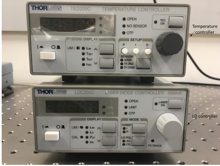
Figure 3.10. LD controller and temperature controller
