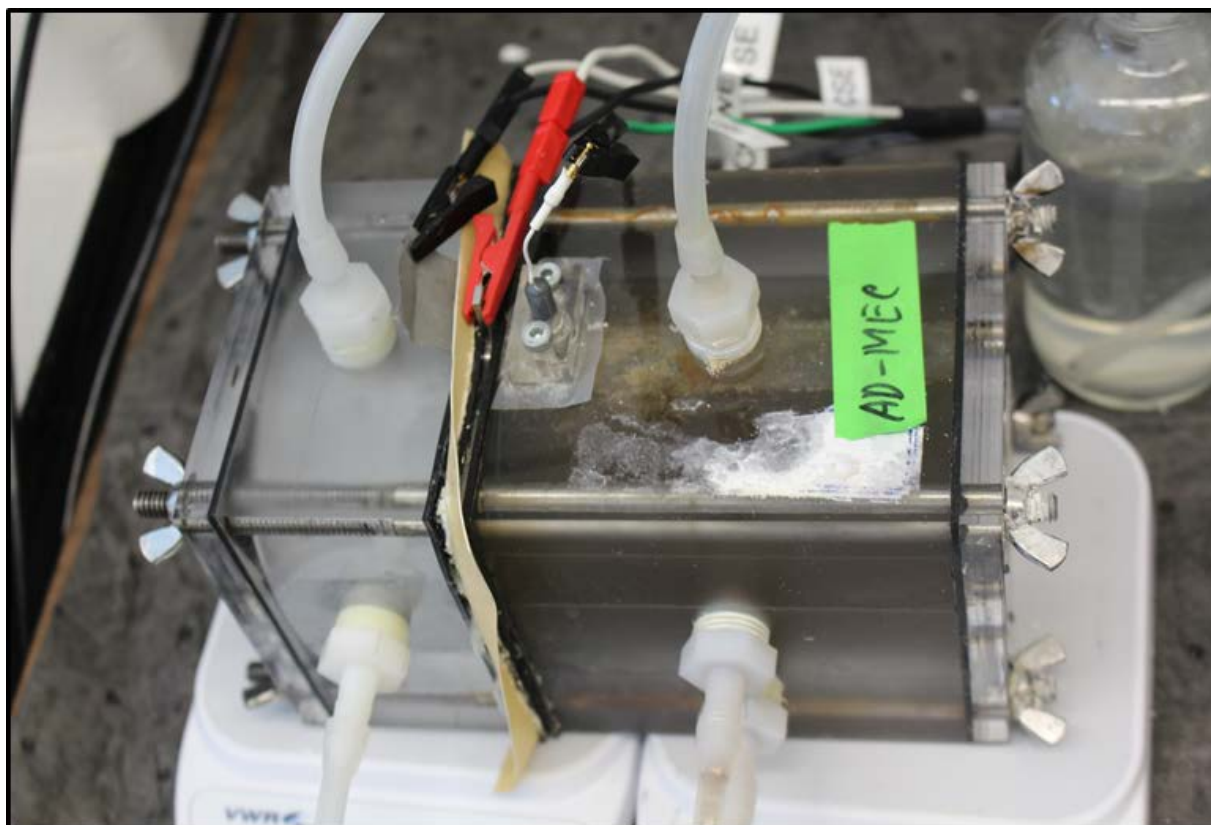
Fig. S1. Photograph of microbial electrolysis cell (MEC) used in this study.
