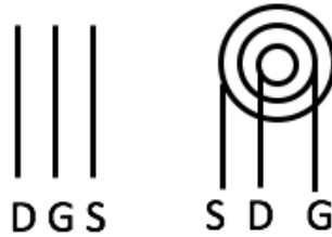
Figure 3.1: Detector design of previous parallel gate MOSkin TM dosimeter and new circular gate MOSkin TM dosimeter
