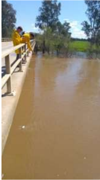
Figure 53: River water sample collection at Wagga Wagga. Sample bottle is hanging on a string to collect water from the centre of the channel.
