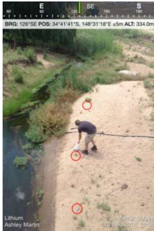
Figure 50: Example of how sediments were collected from river banks. Red circles indicate the different sample aliquots. Sample site shown is Granodiorite catchment A at Cunningham Creek.
