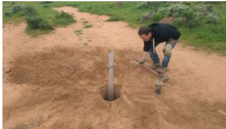
Figure 71: Kerarbury palaeo-channel system, sample N. of Boooroban 1. Aluminium pipe was hammered ~0.55-0.65 m into the ground. Sediments that surrounded the aluminium pipe were removed after hammering.
