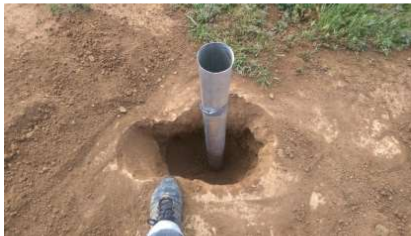
Figure 72: Kerarbury palaeo-channel system, sample N. of Boooroban 2. Aluminium pipe was hammered ~0.65-0.75 m into the ground.
