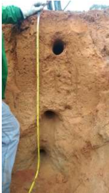
Figure 102: Palaeo-channel samples taken from different depths. Top hole = shallow, centre hole = intermediate, bottom hole = deep. This sample site is Gala Vale.
