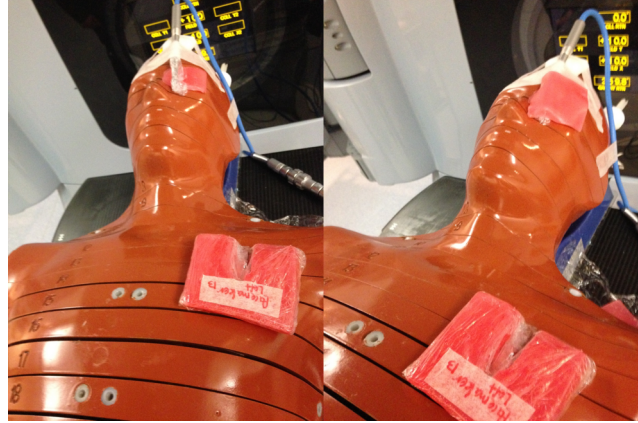
Figure 6.2 Positioning of the ionisation chambers on the anthropomorphic phantom
