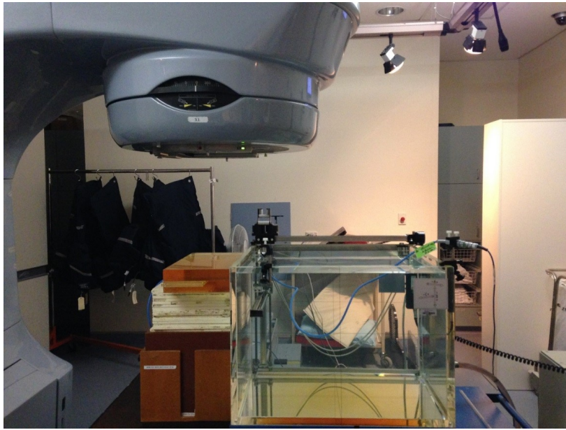
Figure 5.1 Experimental set-up of out-of-field dose measurements, for comparison with the results of Kry et al. (2006) [26]
