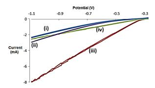
**Figure 1.** Cyclic voltammograms (vs Ag/AgCl) in 0.05 M H<sub>2</sub>SO<sub>4</sub>/0.2 M Na<sub>2</sub>SO<sub>4</sub>, without light illumination, of FTO glass slides having 1 cm<sup>2</sup> active geometric area, coated with: (i)-(ii) nano-Ni/rGO (ratio 125 mg nano-Ni : 6 mg rGO), (i) immediately after preparation and (ii) after 15 scans; or: (iii)-(iv) 100 nm of sputter-coated Pt, (iii) immediately after preparation and (iv) after 15 scans. Scan rate: 5 mV/s.
