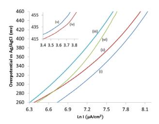
**Figure 9.** Tafel plots for: (i) PEDOT/nano-Ni/rGO containing 125 mg nano-Ni and 5.4 mg rGO (with light illumination), (ii) PEDOT/nano-Ni/rGO containing 125 mg nano-Ni and 5.4 mg rGO (without light illumination), (iii) control nano-Ni/rGO (without PEDOT) containing 125 mg nano-Ni and 5.4 mg rGO (with light illumination), (iv) control PEDOT only (with light illumination), (v) control PEDOT only (without light illumination), and (vi) control bare Pt.
