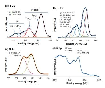
**Figure 7.** X-ray photoelectron spectroscopy (XPS) of PEDOT/Nano-Ni/rGO containing 125 mg nano-Ni and 5.4 mg rGO, showing measured data (individual data points) and modelled data (solid black lines) for the: (a) S 2p, (b) C 1s, (c) O 1s, (d) Ni 2p spectra.
