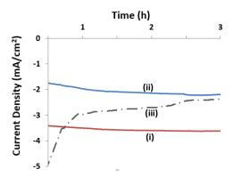
**Figure 4.** Chronoamperograms at -0.75 V (vs Ag/AgCl) in 0.05 M  $H_2SO_4/0.2$  M  $Na_2SO_4$  of FTO glass slides coated with: (i) PEDOT/nano-Ni/rGO (125 mg nano-Ni/5.4 mg rGO; with light illumination), (ii) nano-Ni/rGO without PEDOT (control) (125 mg nano-Ni/5.4 mg rGO; with light illumination), and (iii) bare Pt (control) (without light illumination).
