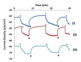
Figure 2. Chronoamperograms at -0.75 V (vs Ag/AgCl) in 0.05 M  $\rm H_2SO_4/0.2~M~Na_2SO_4$ , after 3 h of operation, with and without light illumination (0.25 sun), of FTO glass slides coated with: (i) PEDOT alone, (ii) PEDOT/nano-Ni (125 mg nano-Ni), and (iii) PEDOT/rGO (5.4 mg rGO) (\*='light on', #='light off). Note that the data in graph (b) is in mA/cm² and therefore substantially larger than the data in graph (a), which is in  $\mu A/cm^2$ .
