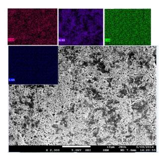
**Figure 5.** (a) Scanning electron microscope image of PEDOT/Nano-Ni/rGO containing 125 mg nano-Ni and 5.4 mg rGO. The inset images show the elemental distributions, using EDX, of: (b) O, (c) Ni, (d) C, (e) S, and (f) O, Ni, C, S together.
