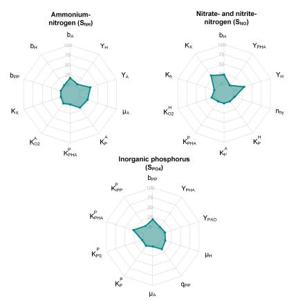
**Figure 2.** Ten most significant parameters influencing the variability of ammonium-nitrogen, nitrateand nitrite-nitrogen, and phosphate in the activated sludge (AS) systems. The results in the radar graphs are the proportion of sensitivity function ( $s_{ij}$ ) for the state variable against the changes of each model parameter over the total sum of sensitivity measures. The description of the influential parameters in the graph can be found in the Supplementary Material F.
