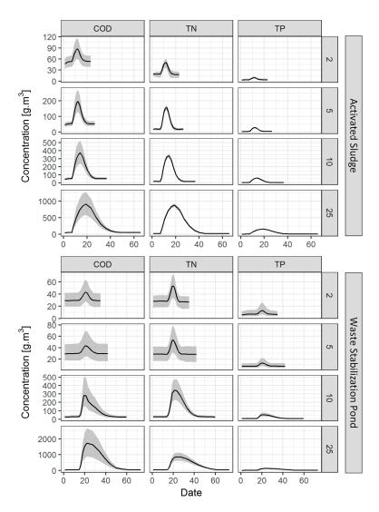
**Figure 5.** The performance of the activated sludge (AS) and waste stabilization pond (WSP) under four shock-load scenarios with different wastewater strengths, i.e., 2, 5, 10, and 25 times higher than the standard OECD domestic wastewater. The lines represent the mean value of the effluent concentrations regarding COD, TN, and TP. The grey bands represent the uncertainty range using 10th and 90th percentile values of the Monte Carlo simulations with all prior uncertainties.
