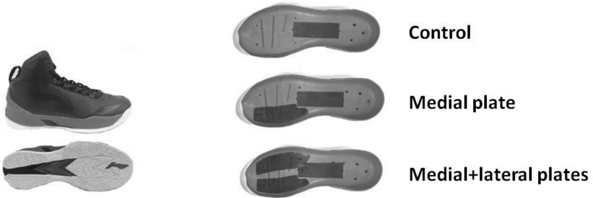
Figure 1 — Test shoe conditions
